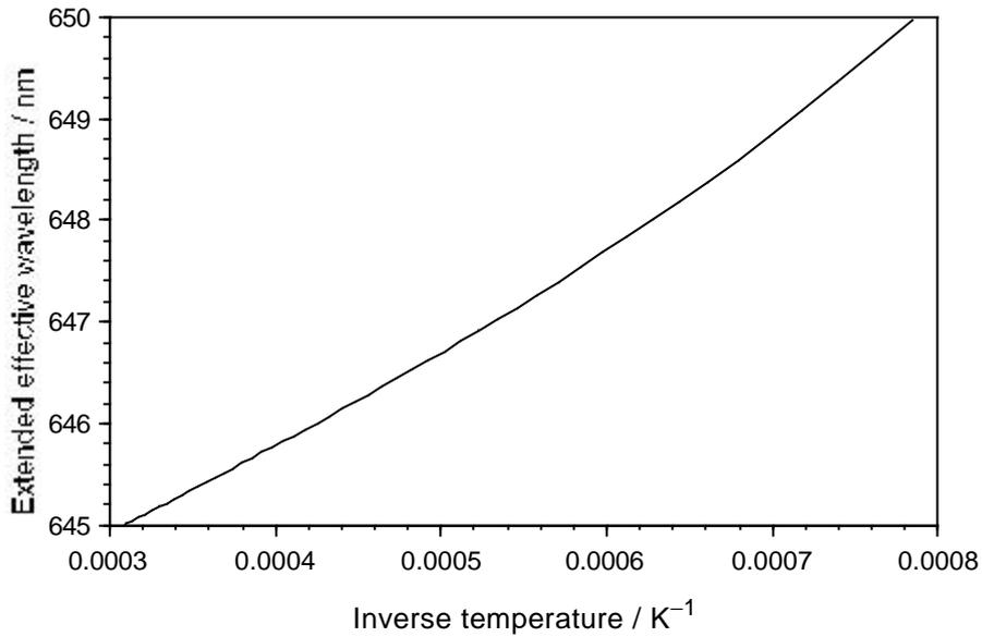
**Figure 3.** Extended effective wavelength as a function of inverse temperature for the spectral responsivity assumed for the calculations. There is clearly some curvature over the relatively large temperature range used.
