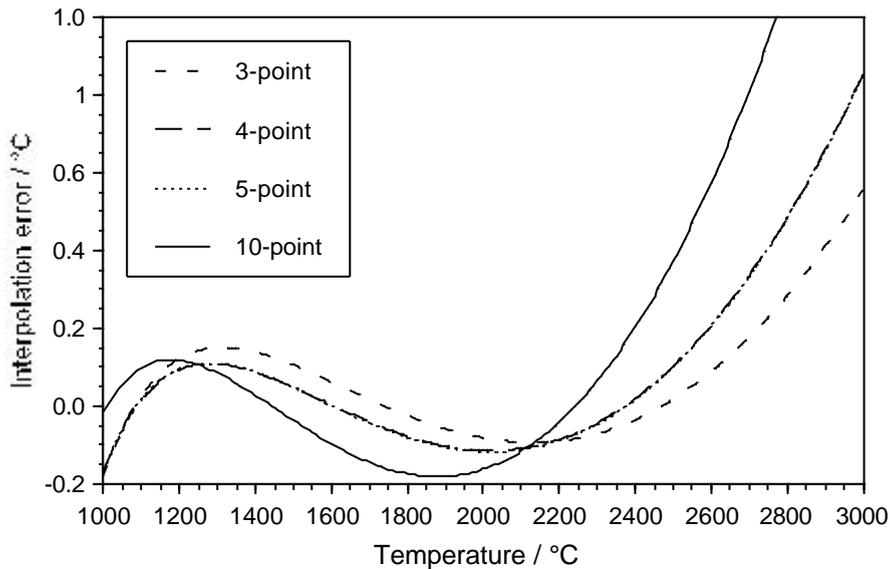
**Figure 2.** The interpolation error for each of the data sets for the interpolation equation (14). The curves for the 4- and 5-point data sets are almost identical.
