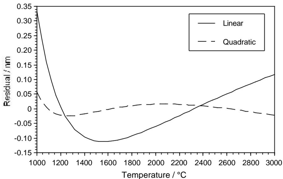
**Figure 4.** Residuals for a linear and a quadratic fit to the extended effective wavelength plotted in Figure 3.
