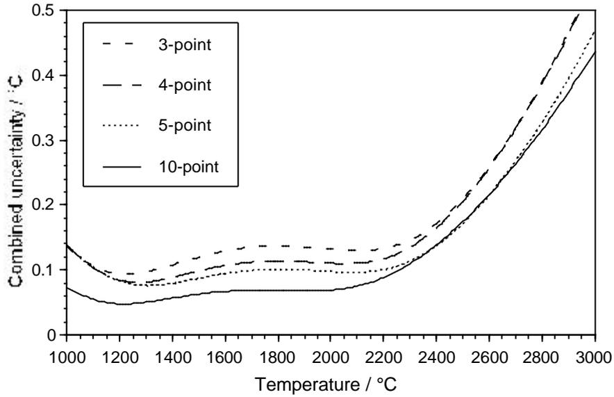
**Figure 1.** Combined uncertainty calculated using equations (6) and (7), with the sensitivity coefficients given by equations (10) and (12), for the 3-parameter interpolation equation (14). The fixed points used for each curve are listed in Table 1. The uncertainties in the temperature of each fixed point is assumed to be 0.1 °C and the uncertainty in each of the measured signals is assumed to be 0.05%.
