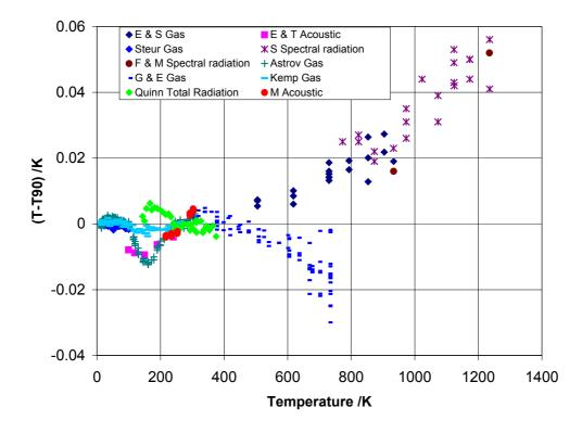
Figure 1: Graph of differences between published thermodynamic temperature determinations from the ITS-90 up to 1235 K (J V Nicholas, 2000). Attributions are as follows.
