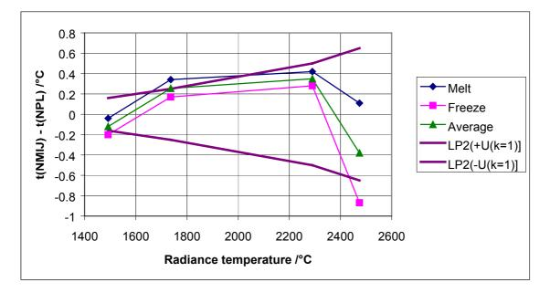
As can be seen the difference in the ITS-90 between the two institutes is very small. The uncertainty curve labelled LP2(U(k=1)) is the one standard uncertainty for the scale realisation of the ITS-90 by NPL using a linear pyrometer (LP2). NMIJ has similar uncertainties so the scale difference is well within the combined uncertainties of the measurements even at the k=1 level.
