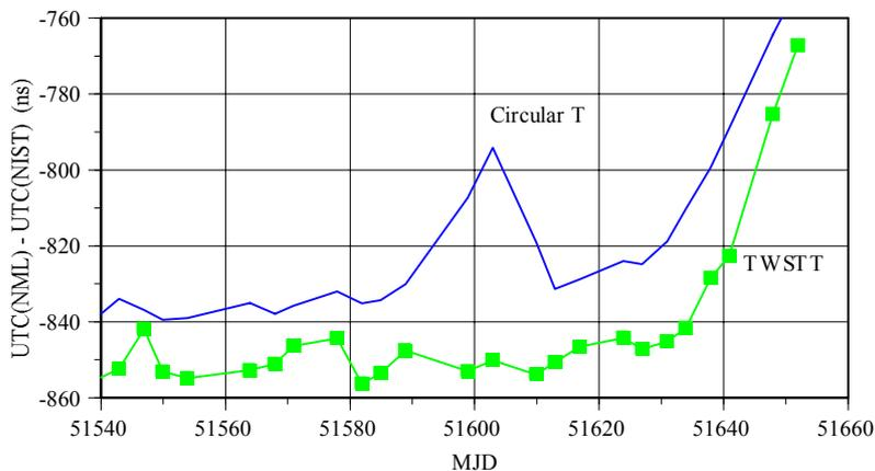
Figure 4: Comparison of UTC(AUS) – UTC(NIST) as calculated from BIPM Circular T and as determined from a TWSTT link between NML and NIST, Fort Collins. The TWSTT data has been offset for clarity.
