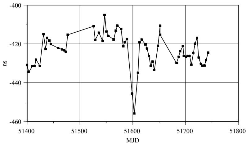
Figure 3: Difference between UTC(AUS) – UTC(NIST) as calculated from BIPM Circular T and UTC(AUS) – UTC(NIST) as determined from a TWSTT link between NML and NIST, Fort Collins.
