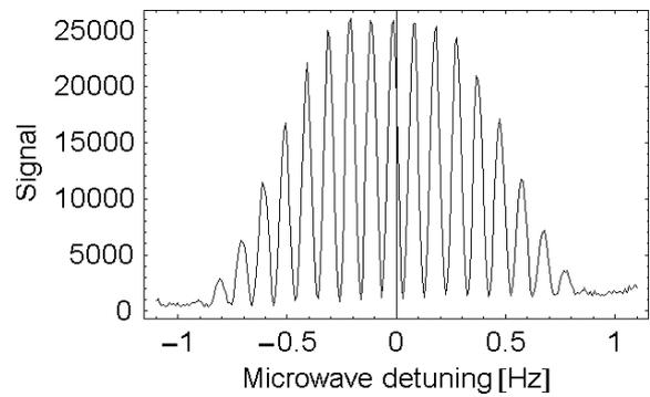
Figure 6: Ramsey fringes recorded for a laser-cooled cloud of  $\sim 10^4$   $^{171}\text{Yb}^+$  ions with a 10 s Ramsey time [3]. A constant background has been subtracted.
