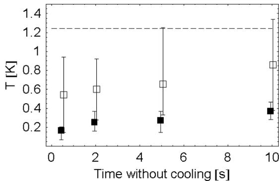
Figure 5: Effective temperature of secular motion as a function of time without laser cooling (see text). The dashed line corresponds to a fractional second-order Doppler shift of  $10^{-15}$ .
