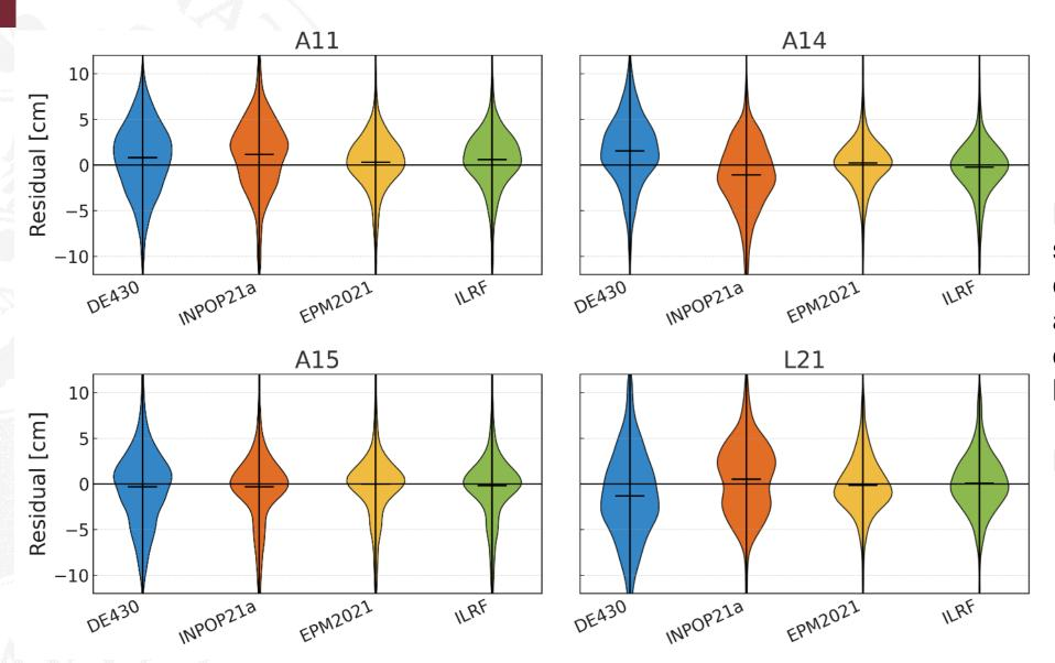
Error distribution for a solution without kinematic corrections (only 3 Euler angles are applied + tidal displacement with VCE-d k<sub>2</sub> value).
