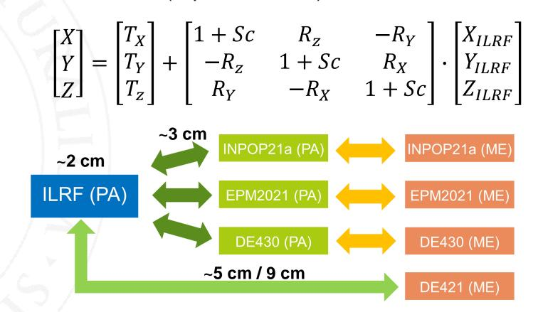
Mean errors of deriving transformation parameters are equal to **3.5**, **2.8**, **and 1.5 cm** for DE430, INPOP21a, and EPM2021, respectively; therefore, the accuracy of the transformation procedure at the level of 2-3 cm is considered sufficient for most of the lunar applications. The tranformation error to ME is **5 cm** (**7-parameters**) or 9 cm (**3-parameters** – rotations only).
