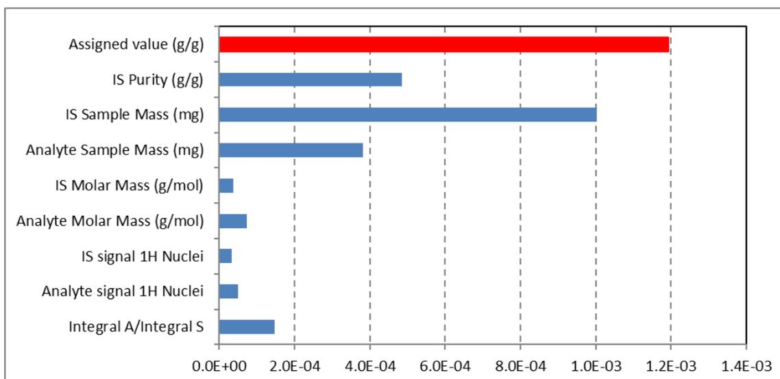
Figure 4 - Relative uncertainty components: DMSO<sub>2</sub> assignment using DSS-*d*<sub>6</sub> in D<sub>2</sub>O.
