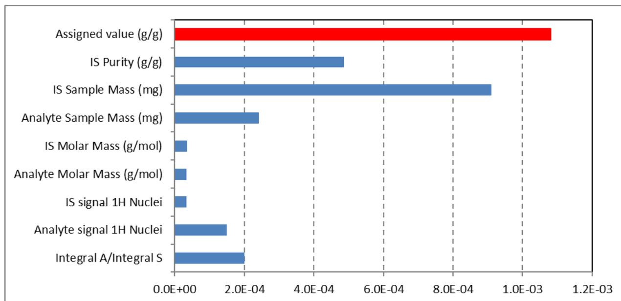
Figure 6 - Relative uncertainty components: MA assignment using DSS- $d_6$  in  $\text{D}_2\text{O}$
