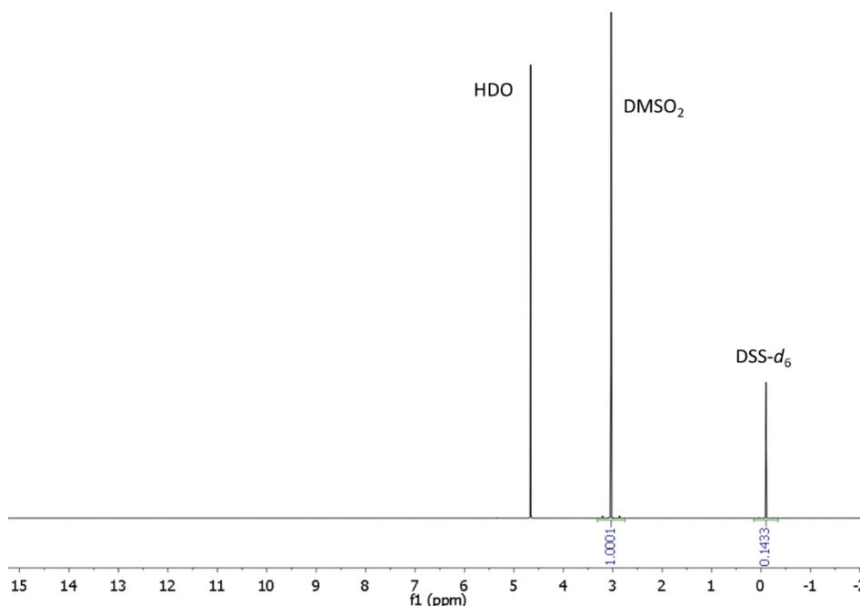
Figure 3 - <sup>1</sup>H NMR spectrum of DSS-d<sub>6</sub> and DMSO<sub>2</sub> in D<sub>2</sub>O.
