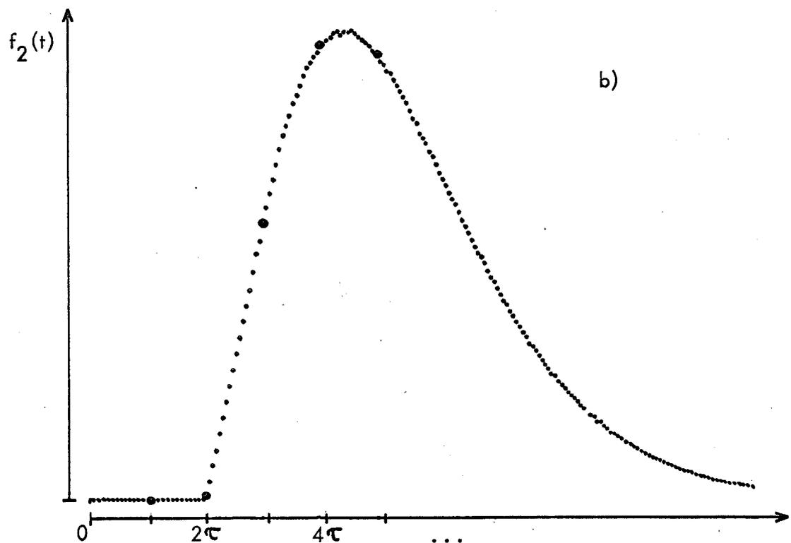
Fig. 3 - Experimental determination of interval densities for an extended dead time (for  $\rho \cong 2.000 \text{ s}^{-1}$ ,  $\tau \cong 400 \mu\text{s}$ ).
