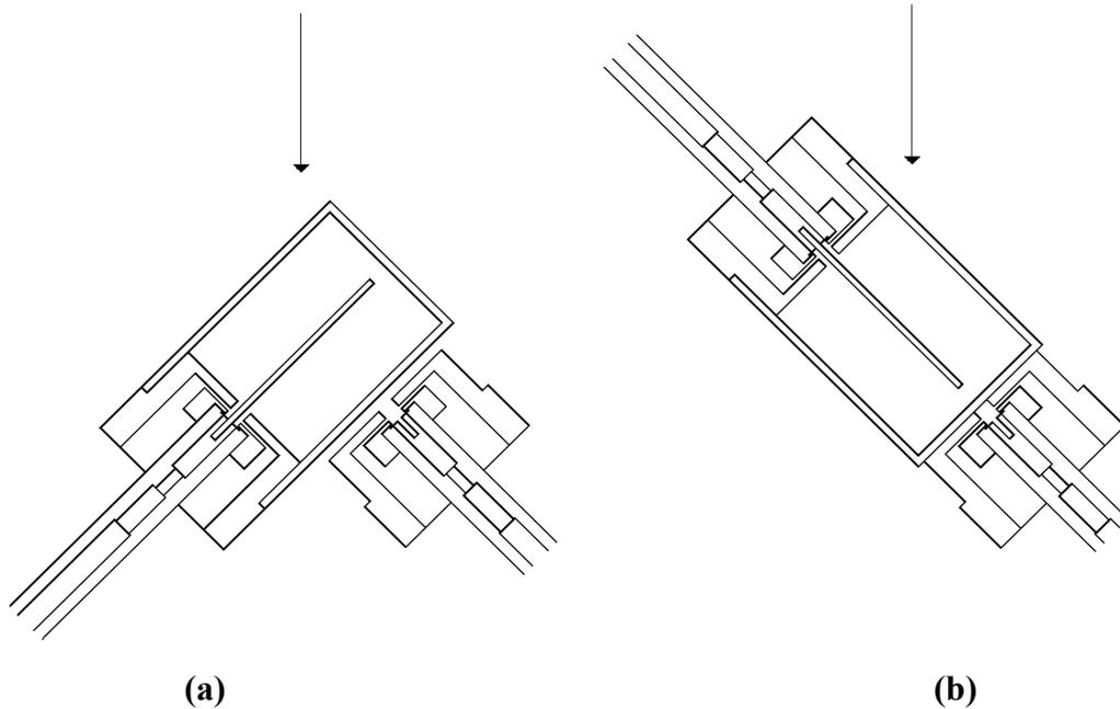
**Figure 3 (a) and (b). Layouts of an ionization chamber and a dummy stem.**
