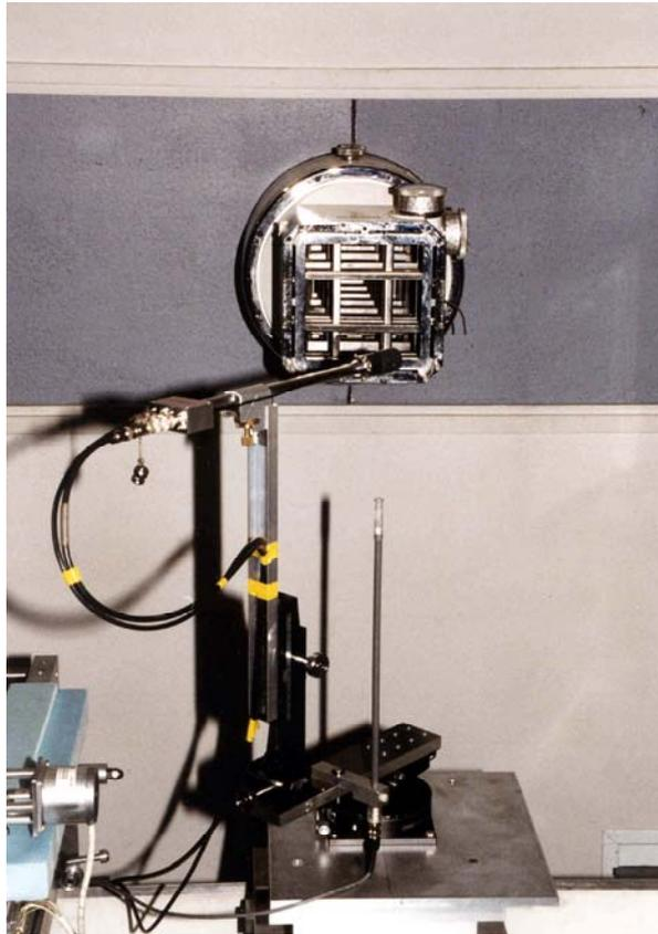
**Figure 1. Photograph of the NMIJ chamber at the reference position in the  $^{60}\text{Co}$  beam**
