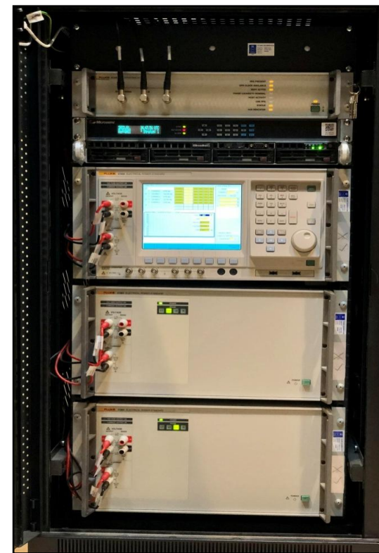
Traceable CSIR-NPL PMU-CAL system
