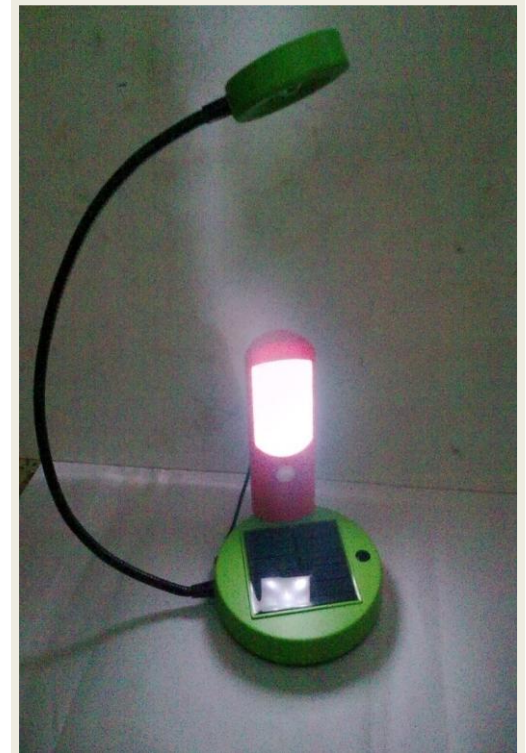
Demonstration of solar lamp with NPL anode & CECRI cathode
