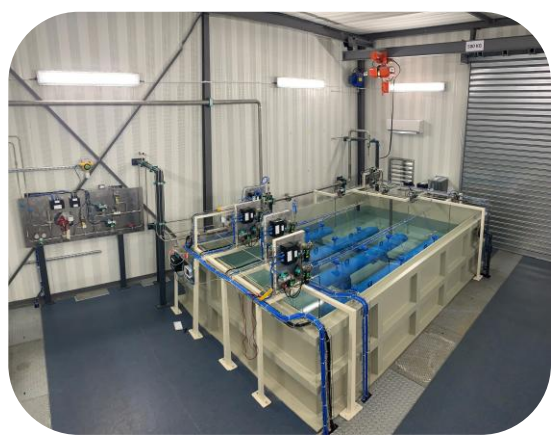
New PVTt facility – CESAME( LNE-LADG) for H 2 , HENG, Air for calibration of sonic nozzles
