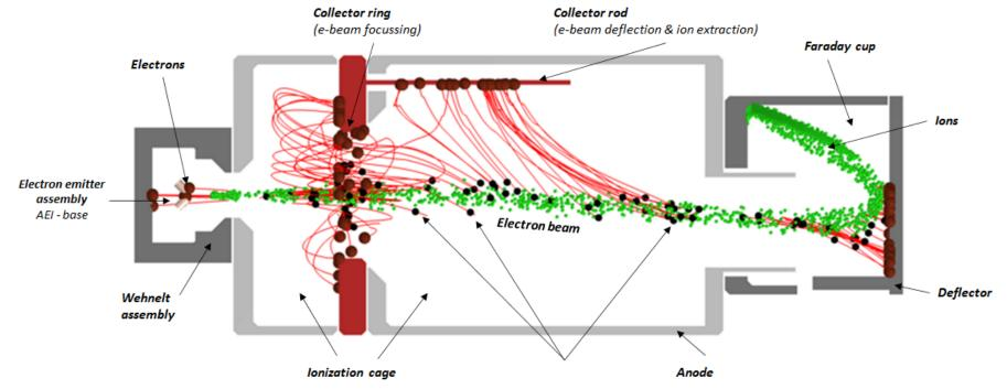
Evaluation and metrological performance of a novel ionisation vacuum gauge suitable as reference standard, Jousten et al, Measurement 210, 31 (2023)
