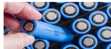
Fig. 2 Illustration of the visual inspection of a 18650 cell .
