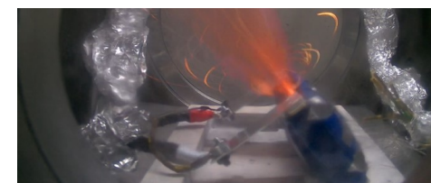
Fig. 4 A snapshot of the moment of thermal runaway failure of a Lithium-Ion cell.
