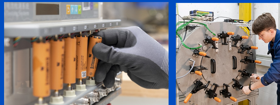
Fig. 1 Lithium-ion cells charging and discharging tests (left) and abuse tests (right)
