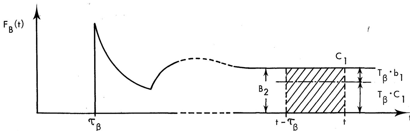
Fig. 2 - Total arrival density for a  $B_2$ -pulse in the vicinity of an original  $C_1$ -event at  $t$ . The origin  $t = 0$  is determined by the arrival of a (registered)  $B_2$ -event.
