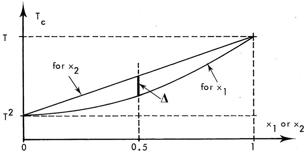
Figure 3 - Schematic graphical plot of  $T_c$  when  $x_1 = C_1/A_1$  or  $x_2 = C_2/A_2$  are used for the abscissa. The difference  $\Delta$  for  $x_1 = 0.5$  and  $x_2 = 0.5$ , indicated in the figure can be readily shown to be  $(T/2) \cdot (1 - T)^2 / (1 + T)$ .
