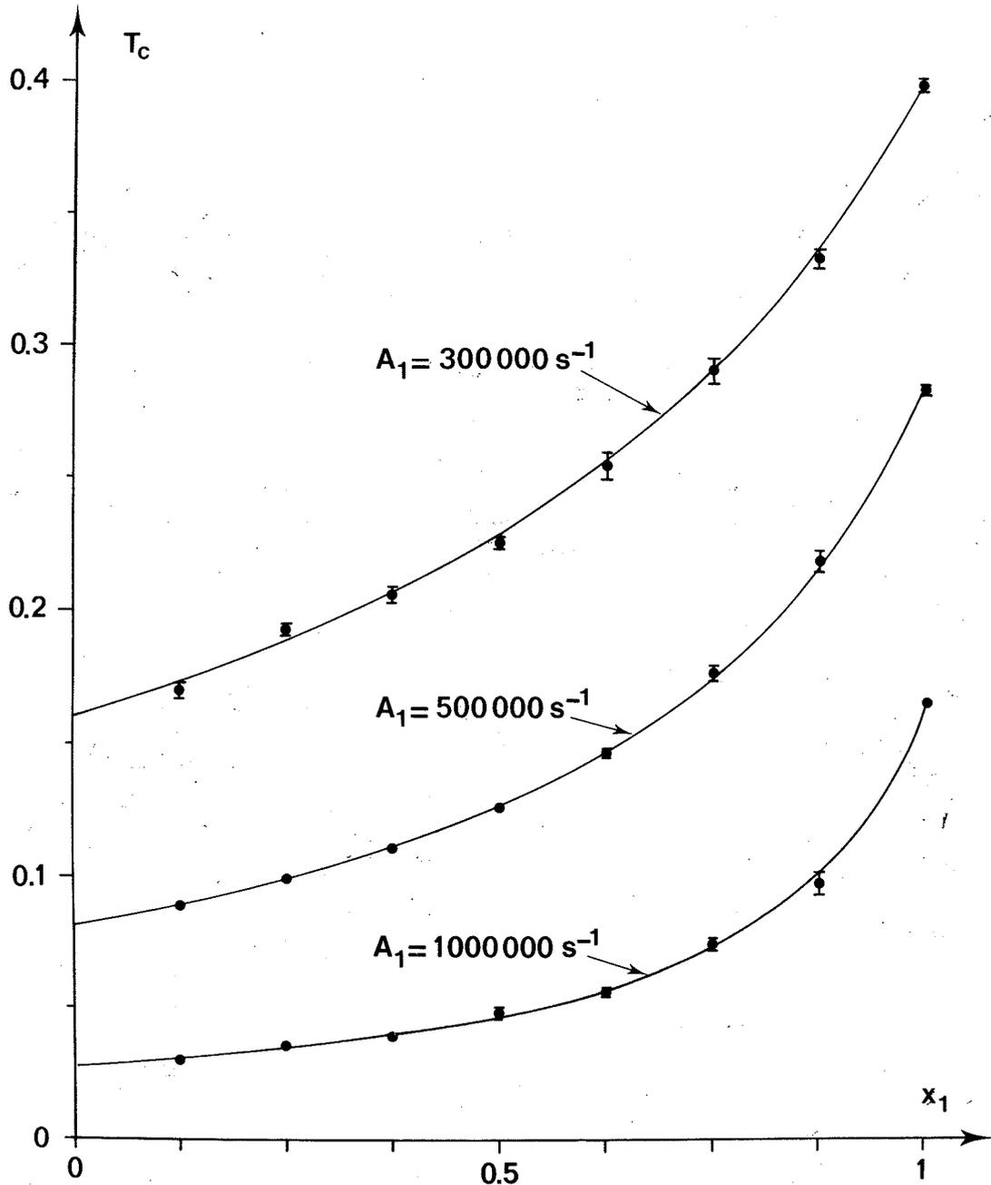
Figure 4 - Result of Monte Carlo simulations for the transmission factor  $T_c = C_2/C_1$  as a function of  $x_1 = C_1/A_1$ . The dead times are always taken as  $\tau = 5\ \mu\text{s}$ . Each experimental point is based on 5 000 registered  $C_2$ -events (only 2 500 for  $A_1 = 1\,000\,000\text{ s}^{-1}$ ). The full line is the theoretical expectation according to (11').
