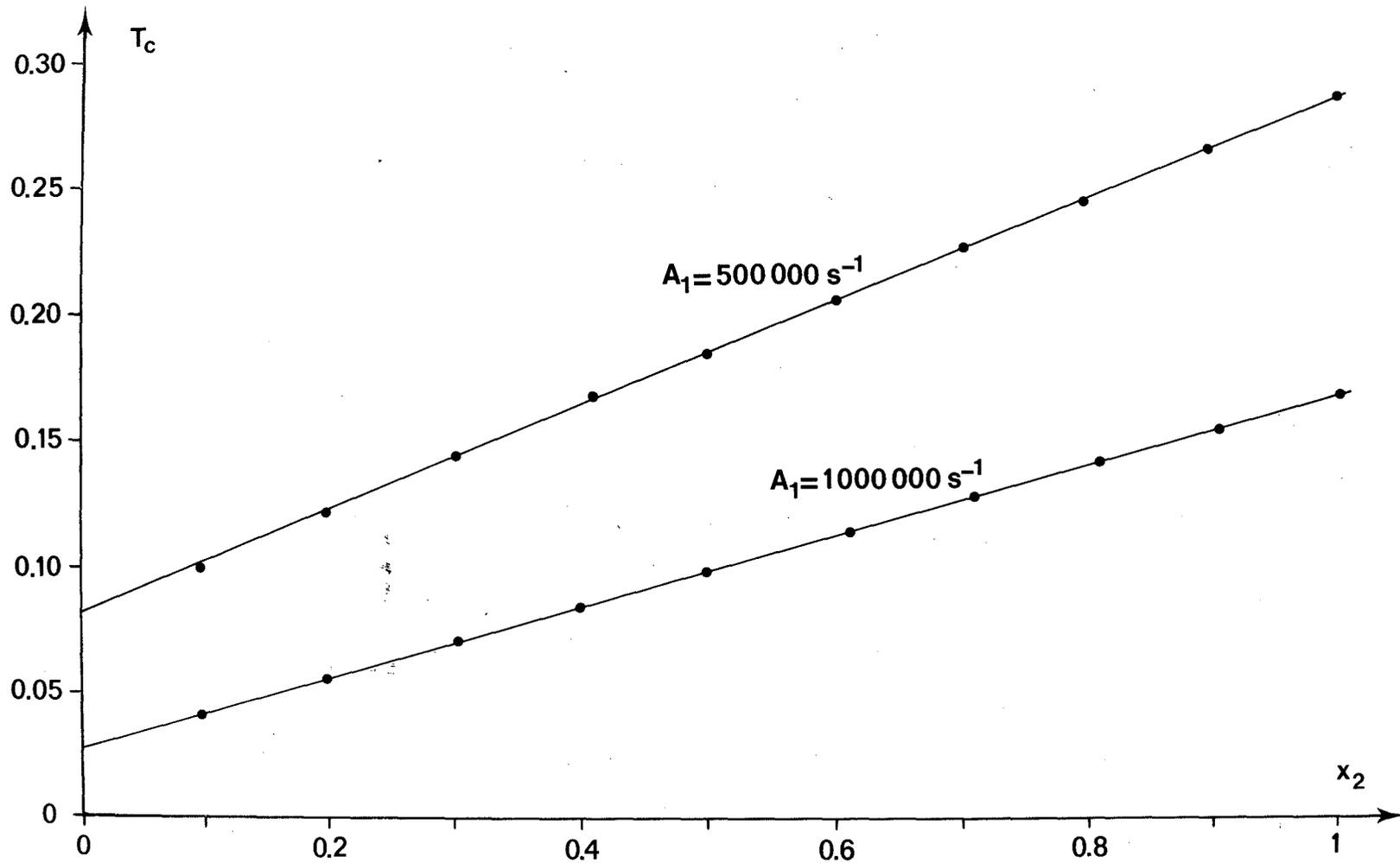
Figure 5 - Similar to Fig. 4, but for the abscissa  $x_2 = C_2/A_2$ , for which theory predicts a straight line given by (12'). For  $A_1 = 500\,000\text{ s}^{-1}$  each point is based on 10 000  $C_2$ -events (but 25 000 for  $A_1 = 1\,000\,000\text{ s}^{-1}$ ). The approximate equidistance of the  $x_2$  values has been obtained by choosing for the input parameter  $C_1$  the values  $A_1 x_2 / [T + x_2(1-T)]$ , with  $x_2 = 0.1, 0.2, \dots, 1.0$ .
