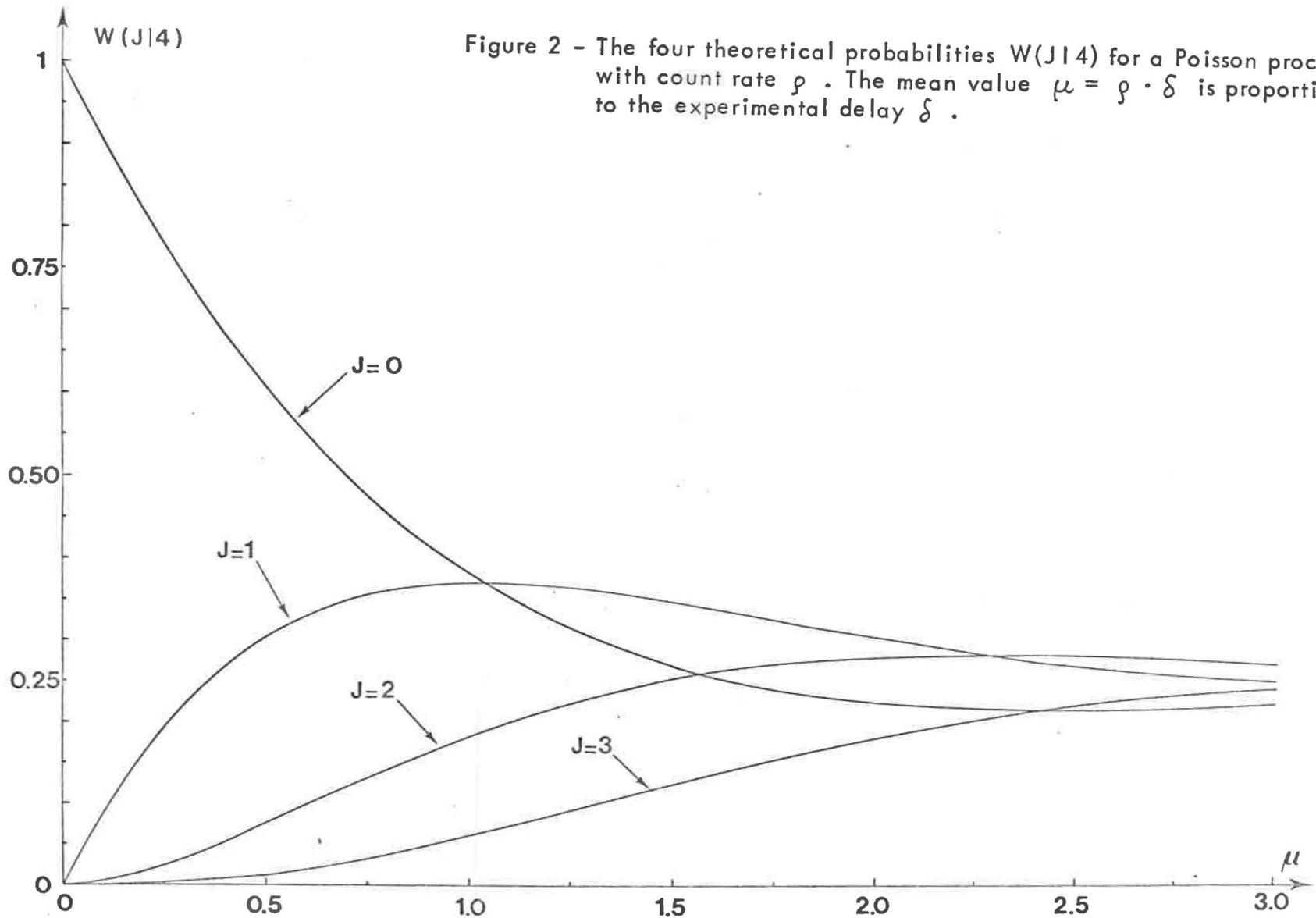
Figure 2 - The four theoretical probabilities  $W(J|4)$  for a Poisson process with count rate  $\rho$ . The mean value  $\mu = \rho \cdot \delta$  is proportional to the experimental delay  $\delta$ .
