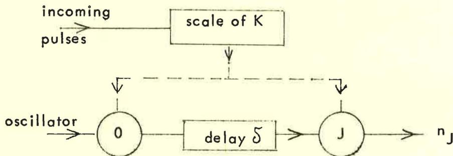
Figure 5 - Final proposal for the experimental arrangement to measure  $\overline{P}(J|K)$ .
