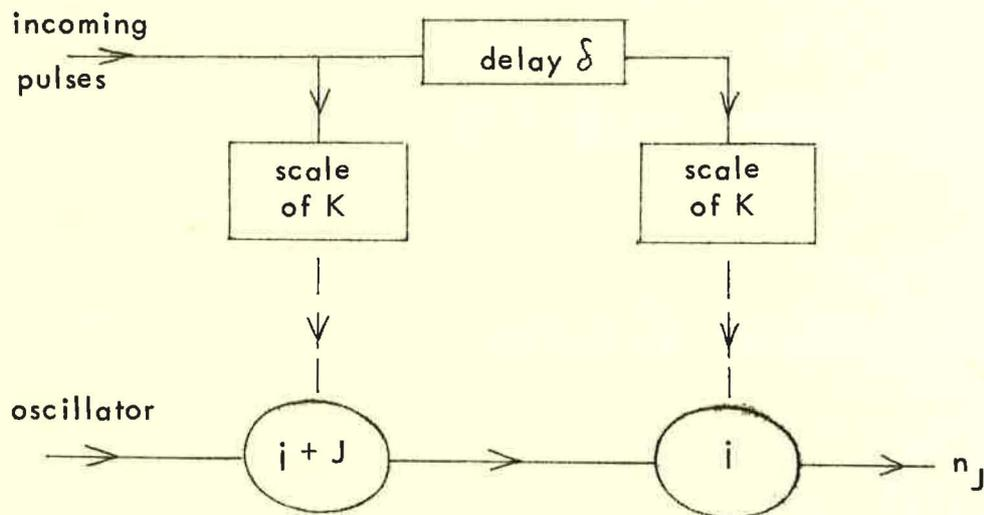
Figure 4 - Simplified schematic arrangement for measuring the probability  $\overline{\mathcal{T}}(J|K)$ .
