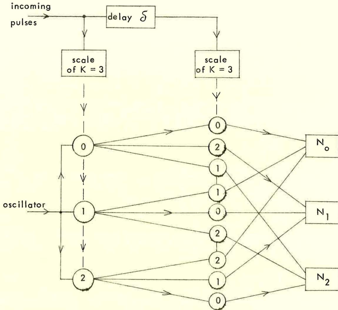
Figure 3 - Schematic diagram for a "complete" correlation measurement with  $K=3$ .
