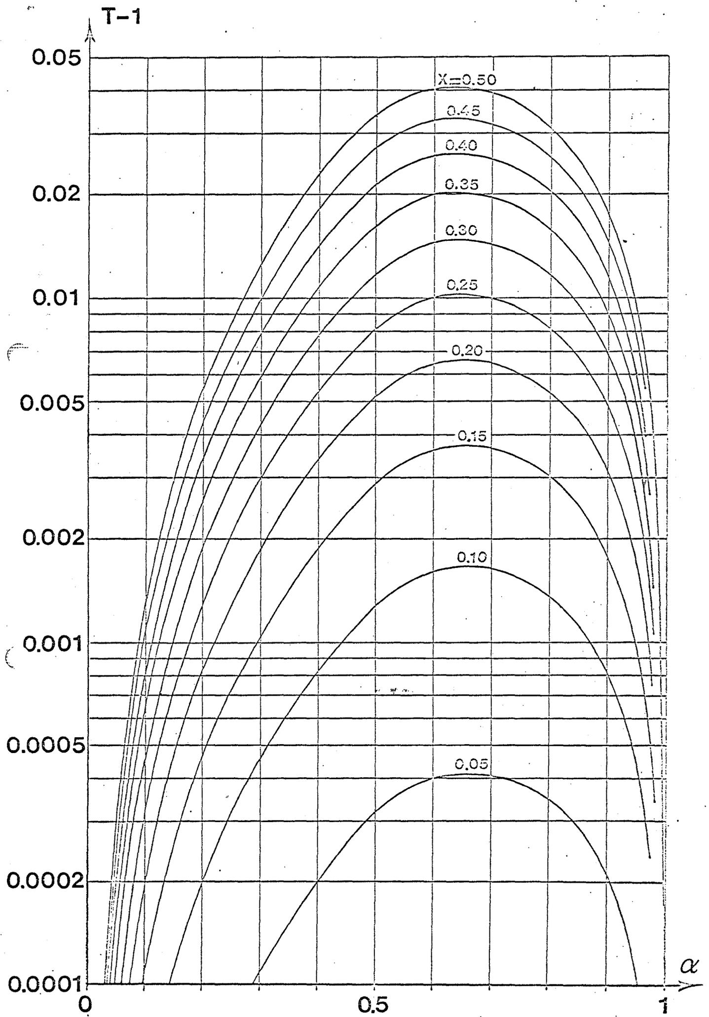
Fig. 2a. - Transmission factor T for x from 0.05 to 0.5
