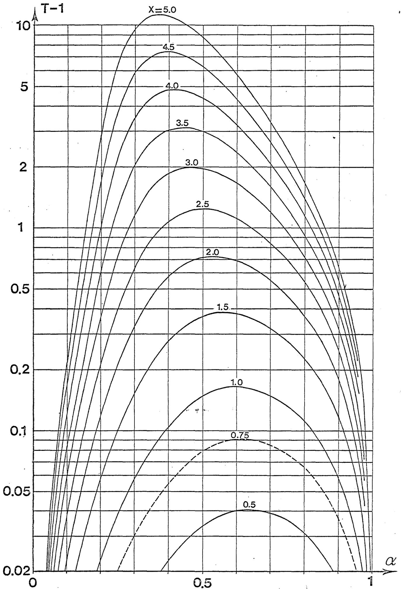
Fig. 2b. - Transmission factor  $T$  for  $x$  from 0.5 to 5.0
