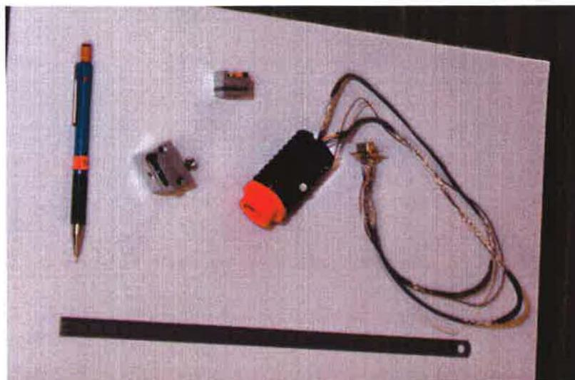
*Figure 2: PTB laser heads*
