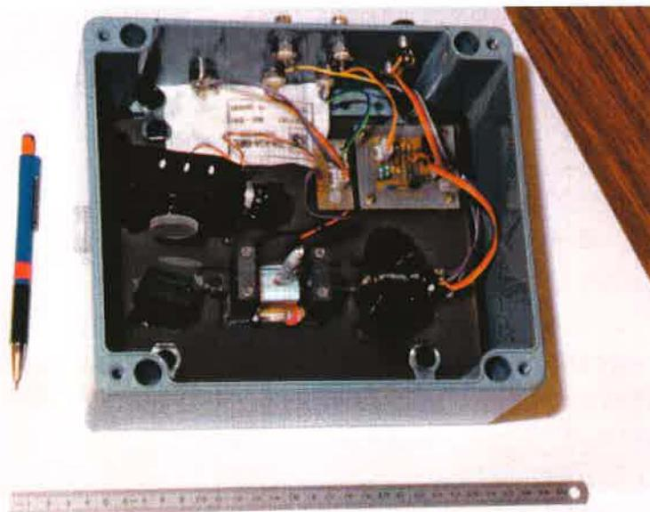
*Figure 1 : DFM ECL Littman configuration with an internal iodine cell*
