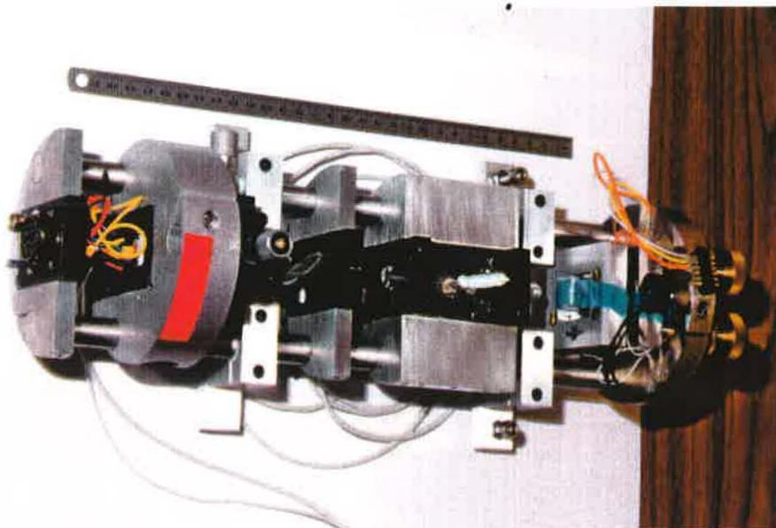
*Figure 3: BIPM ECL (BIREL 1-2) in Littrow configuration with internal iodine cell.*
