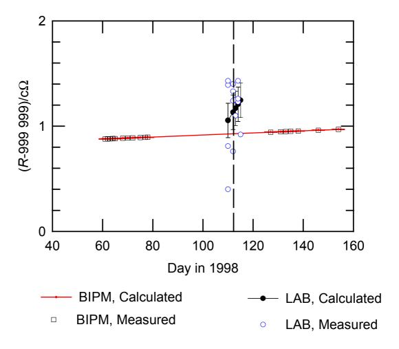
Figure 1. Results of the measurements of BI205 including the BIPM measurements carried out before and after shipping the travelling standard. These results were used in the calculation of the final comparison result. The lines represent the linear least-squares fit to the results of each laboratory. The uncertainty bars represent the type A standard uncertainty. The vertical line near the center represents the mean date of the comparison
