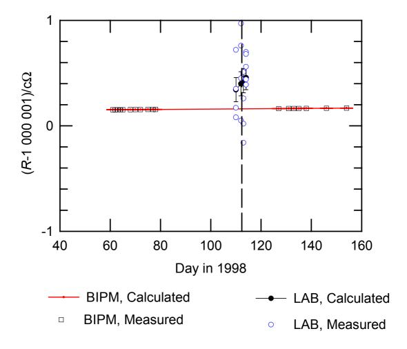
Figure 2. Results of the measurements of BI111 including the BIPM measurements carried out before and after shipping the travelling standard. These results were used in the calculation of the final comparison result. The lines represent the linear least-squares fit to the results of each laboratory. The uncertainty bars represent the type A standard uncertainty. The vertical line near the center represents the mean date of the comparison
