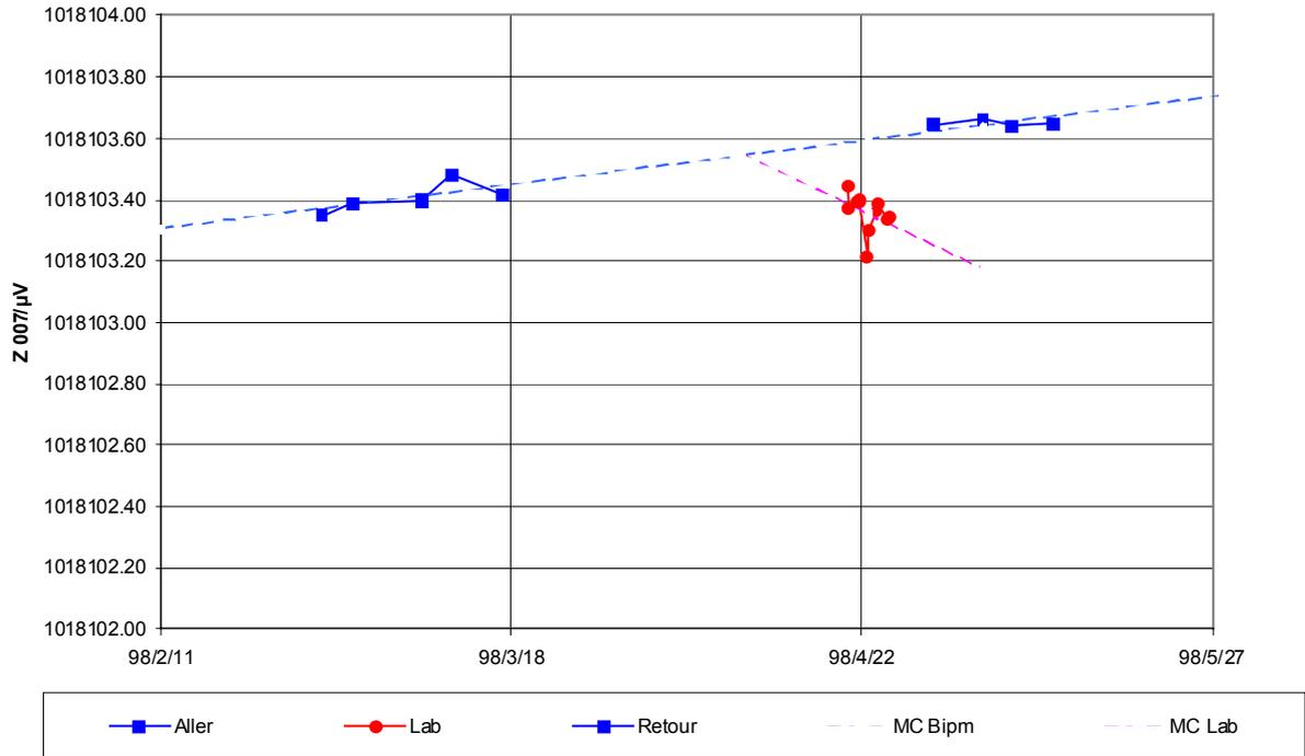
Figure 6. Values assigned to the 1.018 V output of Zener BIPM7 by the NML (Lab) and the BIPM. Dashed lines are the result of linear least-squares fits (MC).
