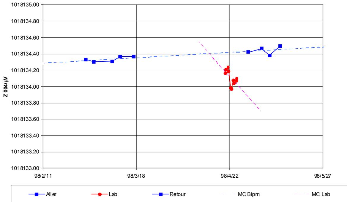
Figure 4. Values assigned to the 1.018 V output of Zener BIPM4 by the NML (Lab) and the BIPM. Dashed lines are the result of linear least-squares fits (MC).
