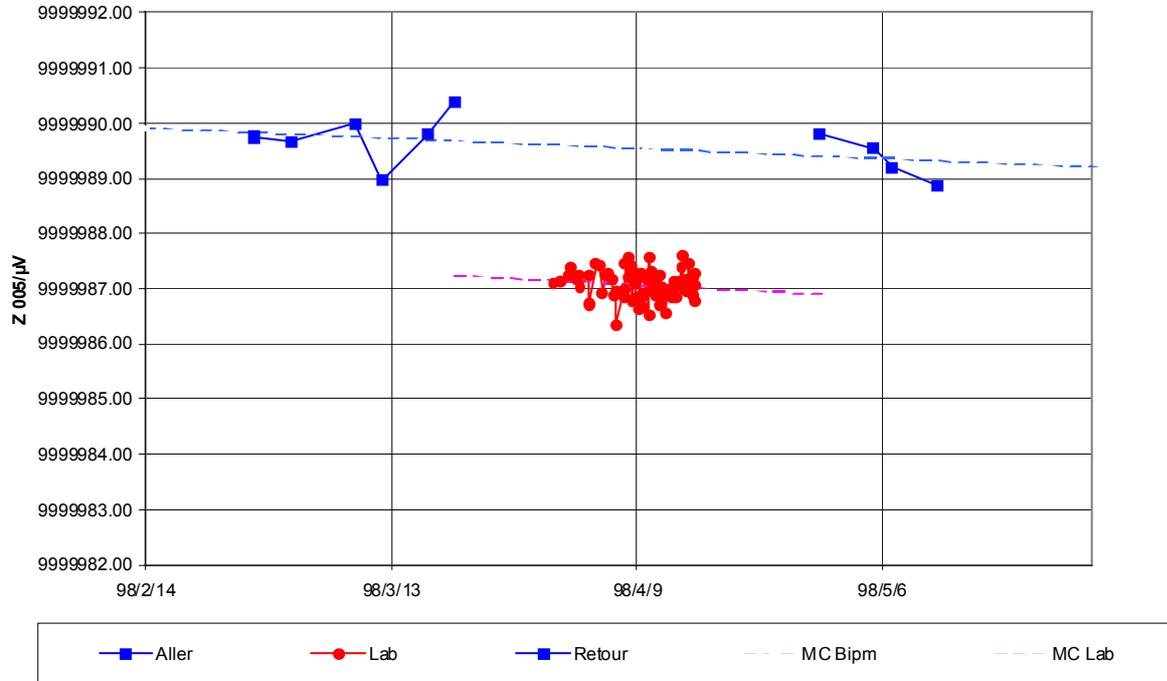
Figure 2. Values assigned to the 10 V output of BIPM5 by the BIPM and the NML during the comparison. The dotted lines are the results of least-squares fits to the BIPM (MC BIPM) and the NML (MC Lab) results.
