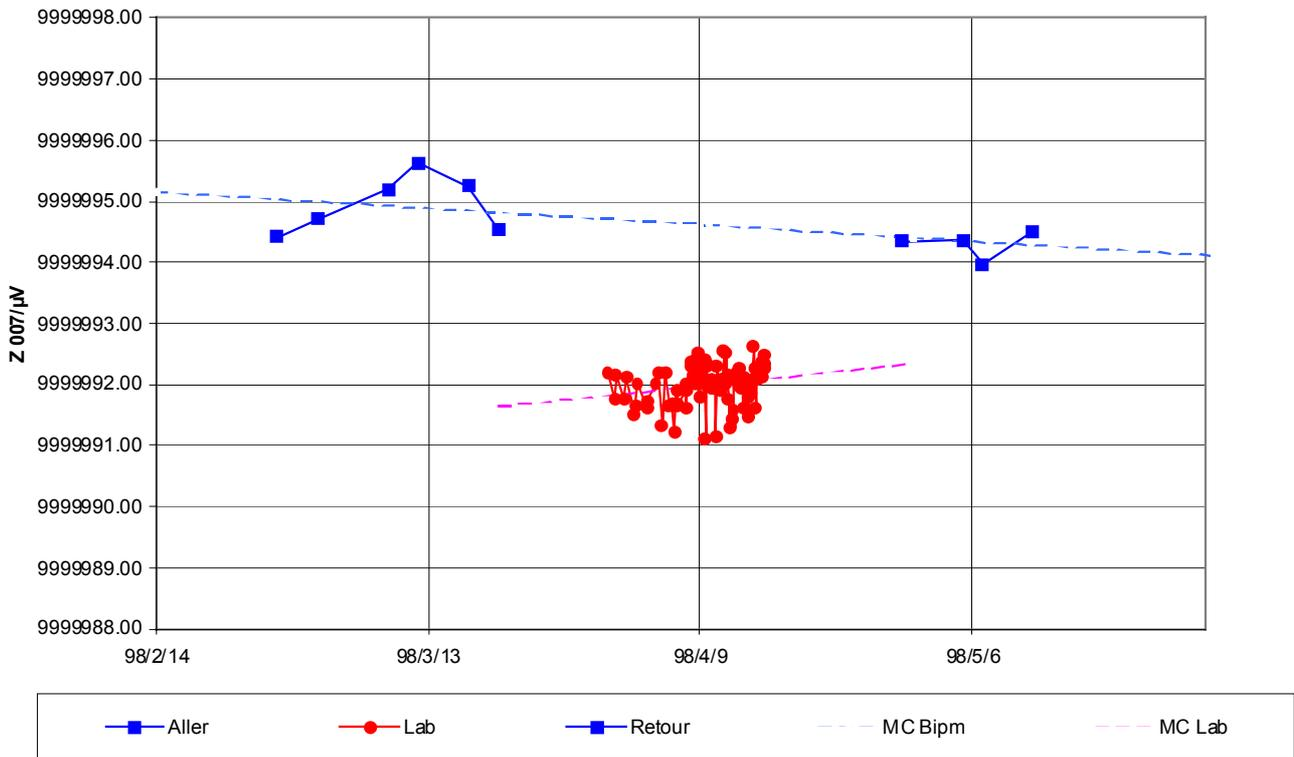
Figure 3. Values assigned to the 10 V output of BIPM7 by the BIPM and the NML during the comparison. The dotted lines are the results of least-squares fits to the BIPM (MC Bipm) and the NML (MC Lab) results.
