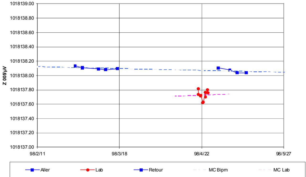
Figure 5. Values assigned to the 1.018 V output of Zener BIPM5 by the NML (Lab) and the BIPM. Dashed lines are the result of linear least-squares fits (MC).
