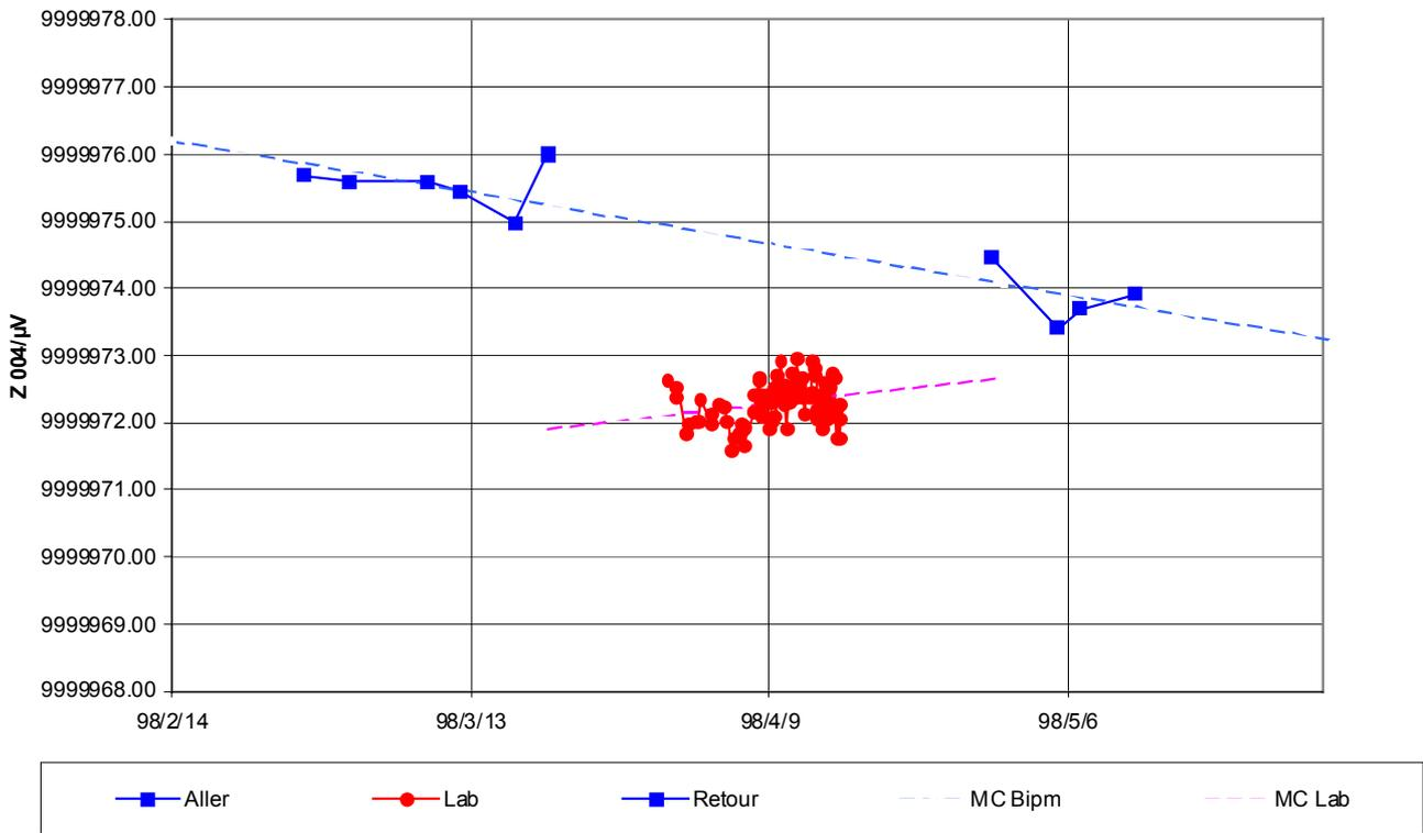
Figure 1. Values assigned to the 10 V output of BIPM4 by the BIPM and the NML during the comparison. The dotted lines are the results of least-squares fits to the BIPM (MC Bipm) and the NML (MC Lab) results.
