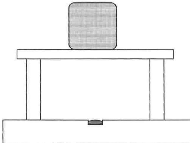
Fig. 1b. Schematic view of induction measurements along the axis of the sample. The distance from the base is set by the height of the bridge.
