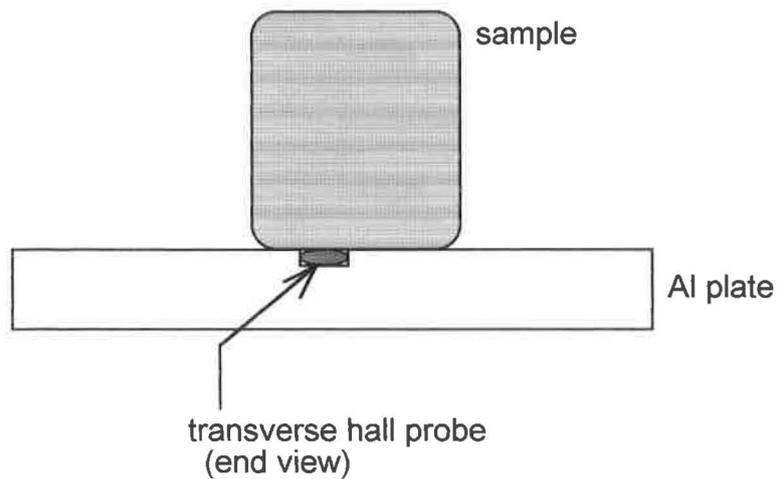
Fig. 1a. Measurement of magnetic induction perpendicular to the base of the sample. The drawing is not to scale. The active area of the probe is about  $1 \text{ mm}^2$ . The top of the aluminium plate is covered with a piece of graph paper whose axes are centred on the active area of the probe. The paper is covered by a single sheet of lens tissue to protect the sample. The sample is displaced relative to the graph paper in order to map out the induction.
