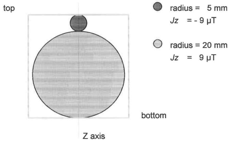
fig. 4. Model of permanent magnetization that accounts qualitatively for induction measurements made on sample 2J. The model assumes that the sample has two regions of permanent magnetization oriented in opposite senses.
