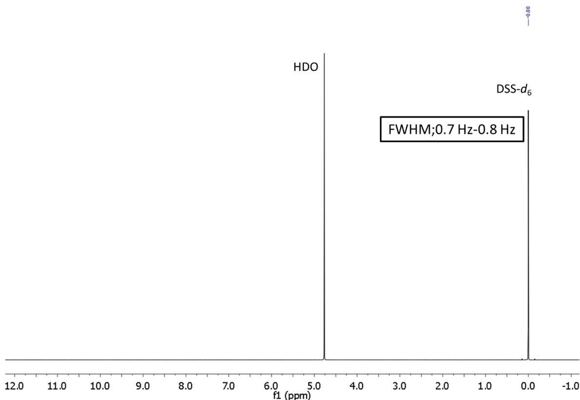
$^1H$  NMR spectrum of DSS- $d_6$  in  $D_2O$ : JEOL ECS-400 spectrometer with Royal probe.
