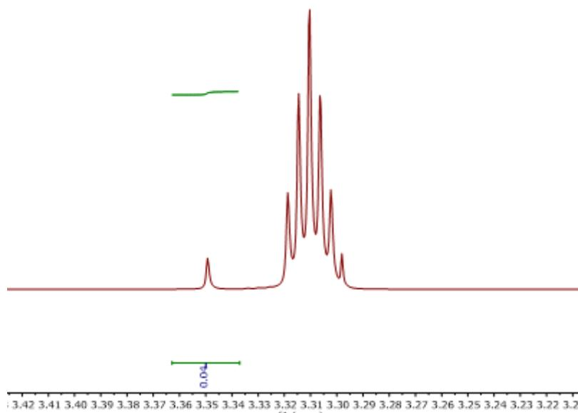
Figure 7 – <sup>1</sup>H NMR spectrum of solvent portion of DMTP in CD<sub>3</sub>OD on storage.
