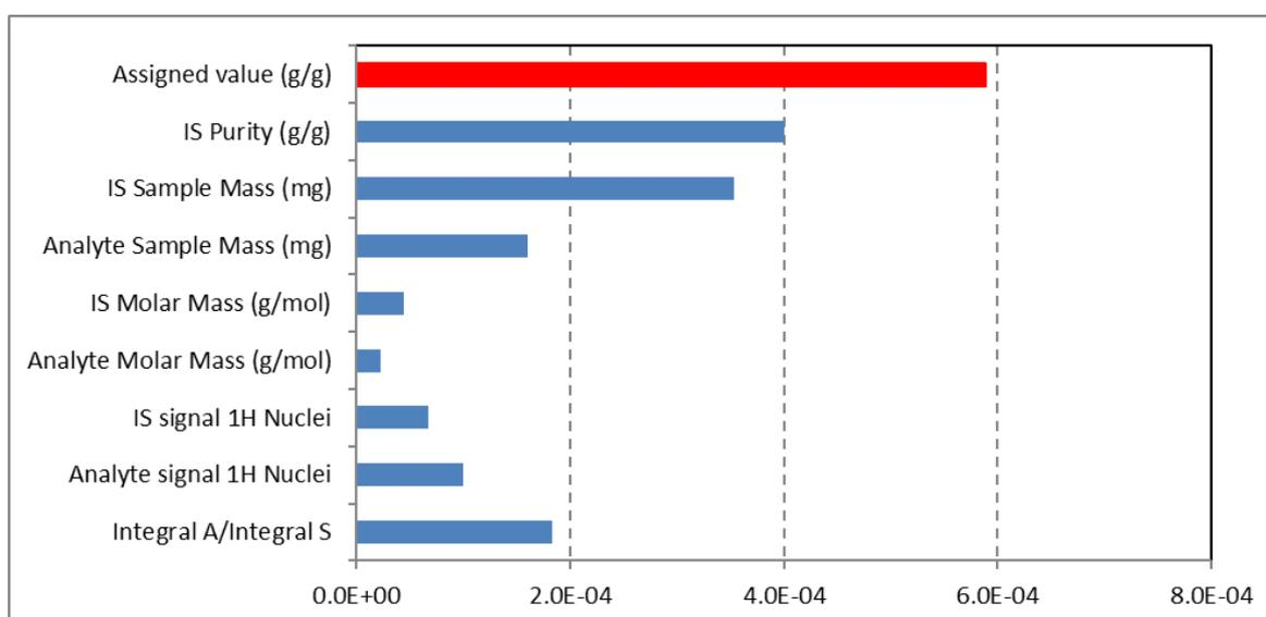
Figure 4 - Relative uncertainty components: BTFMBA assignment using DMTP in  $\text{DMSO}-d_6$
