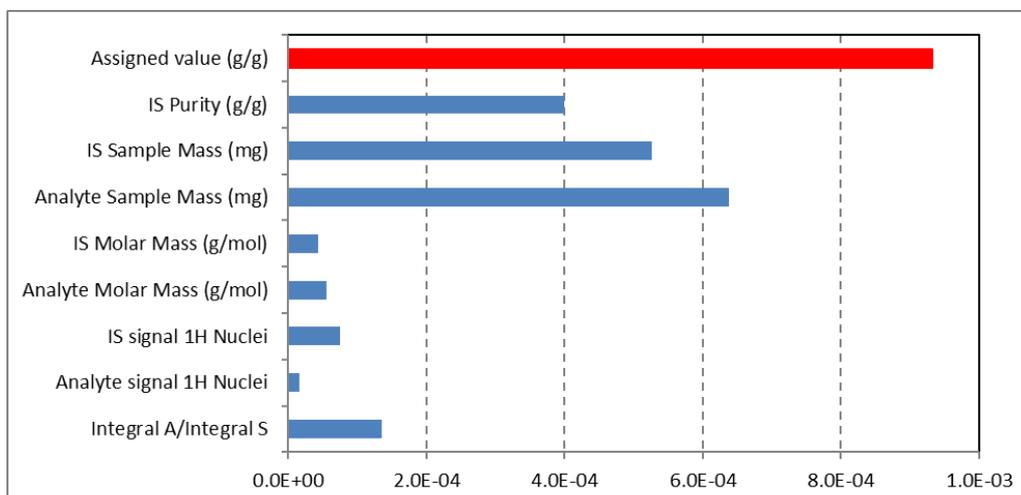
Figure 6 - Relative uncertainty components: BTMSB-*d*<sub>4</sub> assignment using DMTP in CD<sub>3</sub>OD
