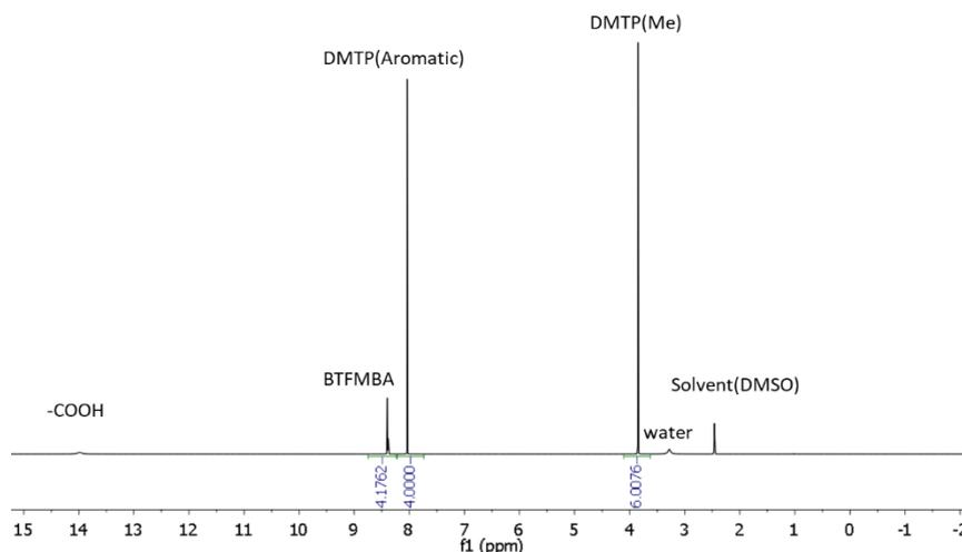
**Figure 3 - NMR spectrum of DMTP + BTFMBA in DMSO-d<sub>6</sub>**
