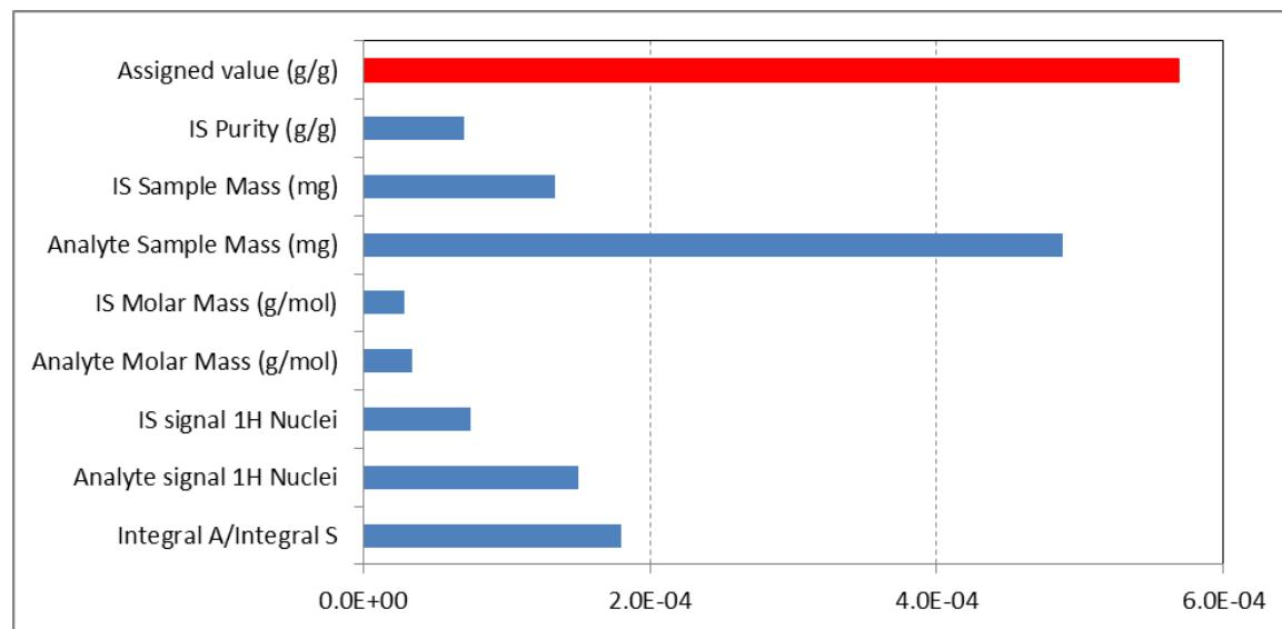
**Figure 4 - Relative uncertainty components (in blue) for the uncertainty in the assigned purity value (in red) for MA using KHP as ISRM in  $\text{D}_2\text{O}$ .**
