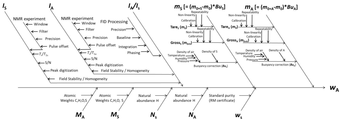
**Figure 2 – Ishikawa diagram for input quantities considered for estimation of the measurement uncertainty of a purity assignment by qNMR**
