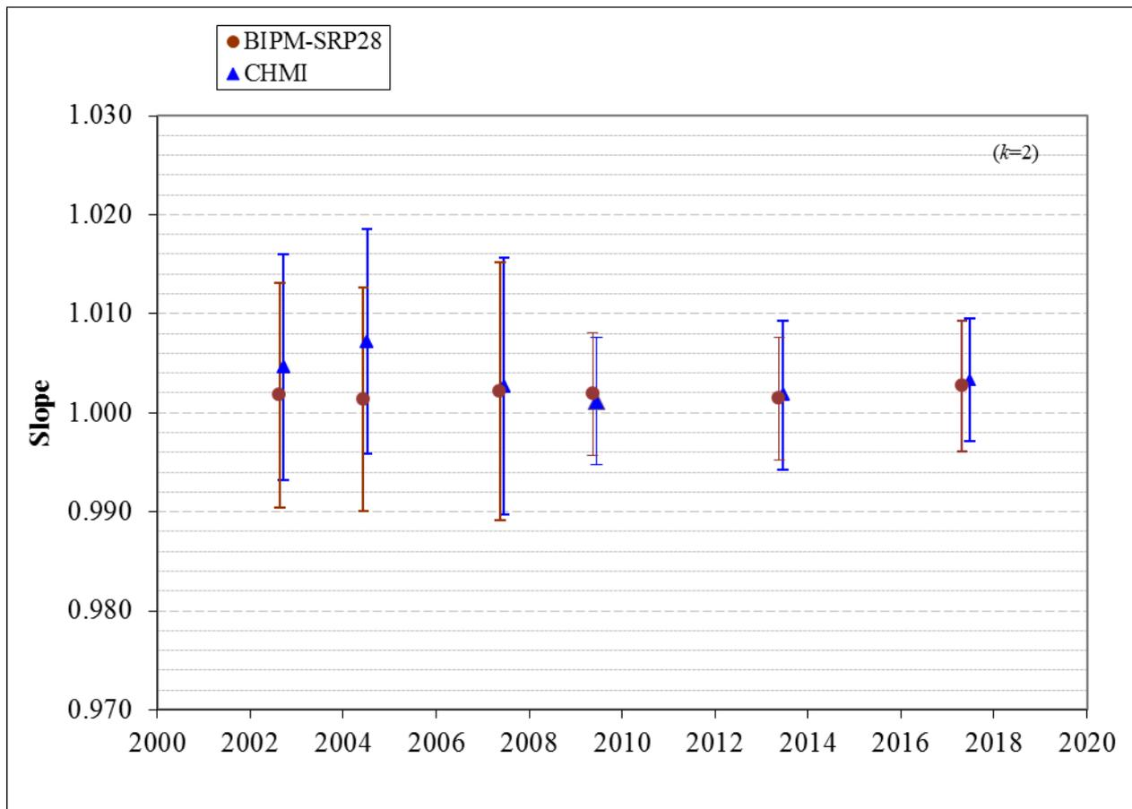
**Figure 2 : Results of previous comparisons between SRP27, SRP28 and CHMI-SRP17 realised at the BIPM. Uncertainties are calculated at  $k = 2$ , with the uncertainty budget in use at the time of each comparison.**
