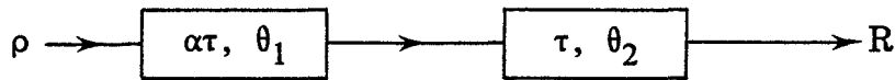
Fig. 1 - Series arrangement of two generalized dead times, with the adopted notation for count rates, dead times and type parameters.
