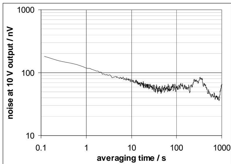
**Figure 2.** Allan variance of the 10 V output of the transfer standard as measured at the VNIIM.
