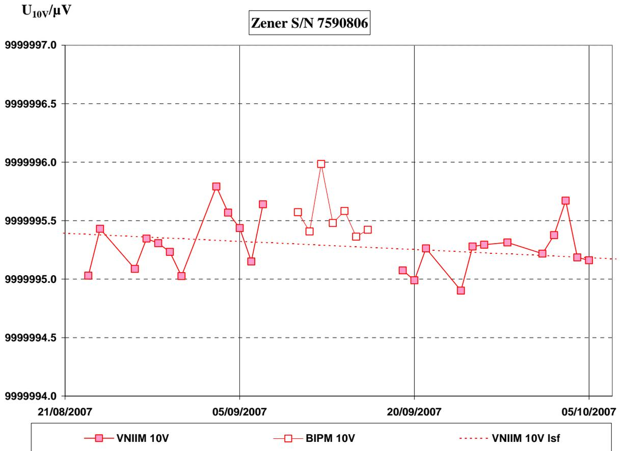
**Figure 1.** Voltage of the VNIIM Zener Standard (S/N 7590806) at 10 V measured at both institutes, as a function of time, with linear least-squares fit to the measurements of the VNIIM.
