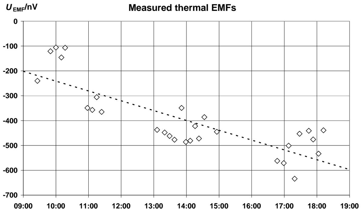
Fig. 3. Measured values of the thermal EMFs during the series of measurements of the BIPM array with the INMETRO system on 11 April. The open diamonds are the thermal EMFs and the dotted line represents the long-term drift.
