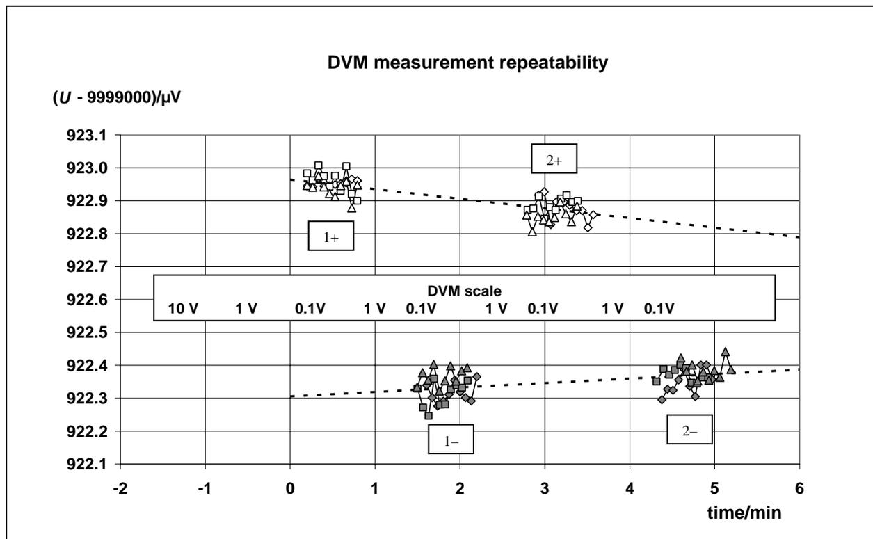
Fig. 2a. Measured values of the BIPM array with the INMETRO system. The open diamonds, squares and triangles are for the measurements in polarity (+) of three series carried out between 10:58 and 11:20 on 11 April; The dark diamonds, squares and triangles are for the measurements in polarity (-). The data are referred to a common time origin corresponding to the beginning of each series.
