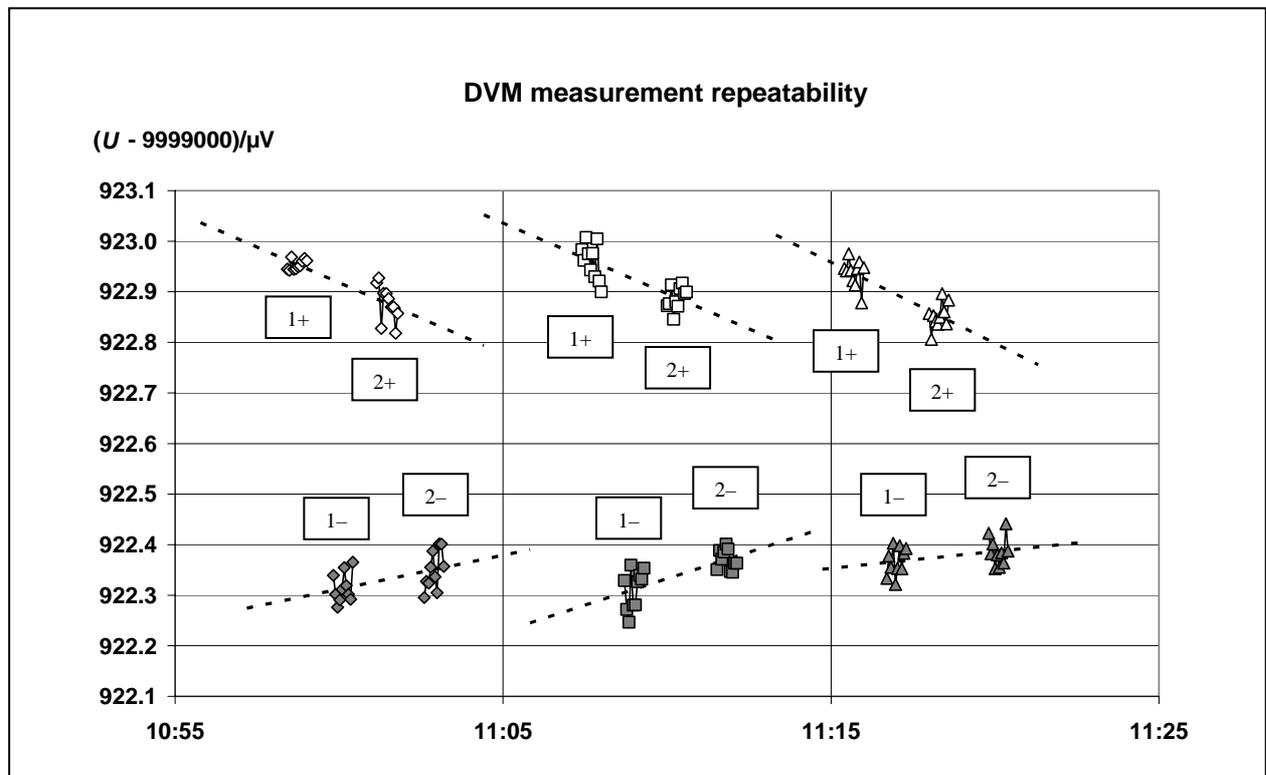
Fig. 2a. Measured values of the BIPM array with the INMETRO system. The open symbols represent the measurements in polarity (+) of three series carried out between 10:58 and 11:20 on 11 April; the filled symbols represent the measurements in polarity (-). The dotted lines show the mean drift of the measured values of the two sets in the same polarity during each series.
