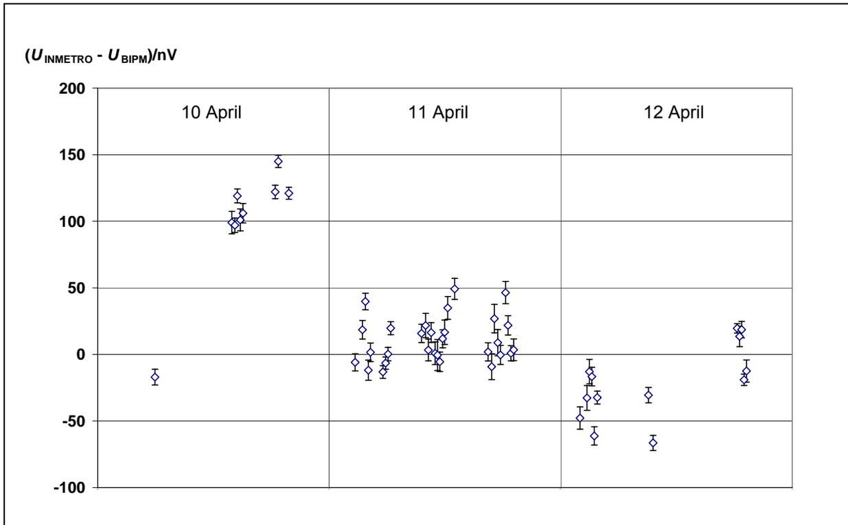
Fig. 1. Difference between the voltage values measured by INMETRO and the corresponding theoretical values of the BIPM array voltage. The error bars are the  $1\sigma$  Type A uncertainties, as computed by the Nistvolt program.
