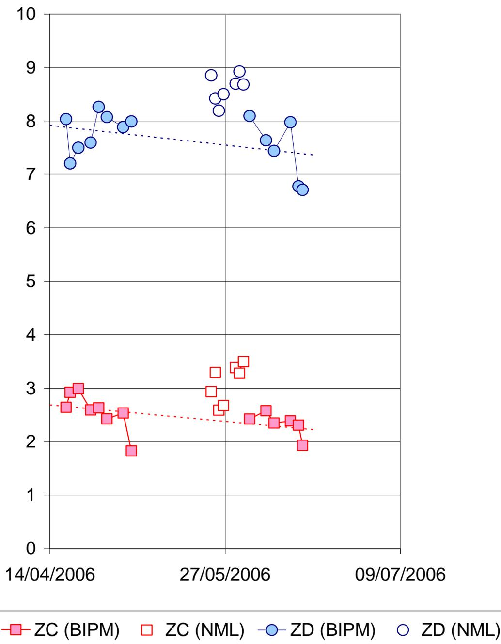
Figure 1. Voltage of BIPM\_C (ZC) and BIPM\_D (ZD) at 10 V, referred to an arbitrary origin, as a function of time, with linear least-squares fit to the measurements of the BIPM.
