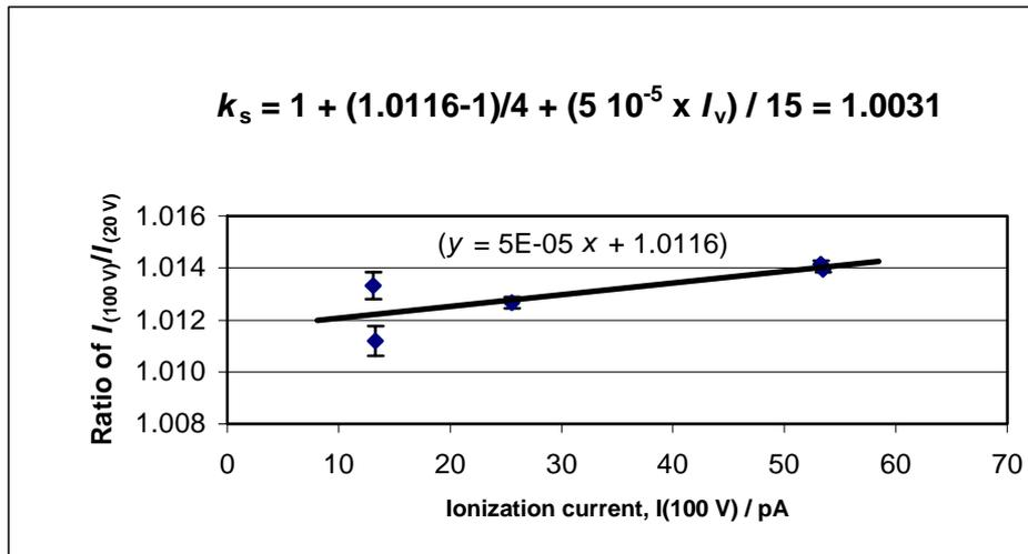
A measurement was made at the BIPM to confirm the effect of an additional stem. This was made while the HRK-3 chamber was in the rotated position. Figure 2 shows the experimental arrangement. The measured effect was of the order of  $5 \times 10^{-4}$  which is similar to that measured at the PTB with the chamber in its normal position.
