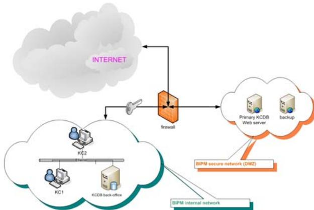
Figure 2. Global architecture of the BIPM network.
