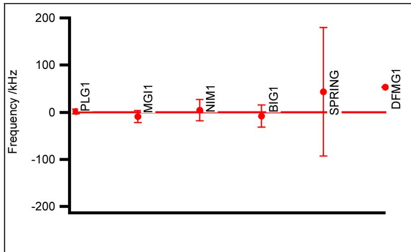
**Figure 1.** Illustration of the dispersion of the measured laser frequencies for the  $b_{10}$  component at a cold finger temperature of 0 °C and a 2 MHz modulation width. The results are given relative to an average frequency for this component (dotted line).
