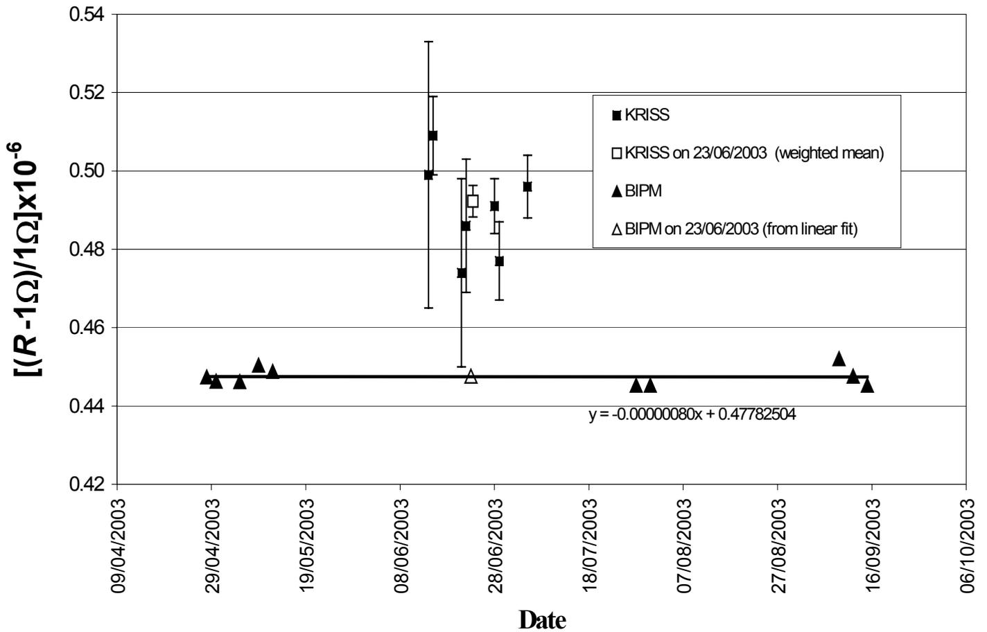
Figure 2. Relative deviation from the nominal  $1 \Omega$  value of the resistance of BIV203 vs time: a linear least-squares fit to the BIPM measurements (full line) and the weighted mean of the KRISS measurements. Uncertainty bars correspond to standard uncertainties of type A only. For each individual BIPM result, the type A standard uncertainty is about 3 parts in  $10^9$ .
