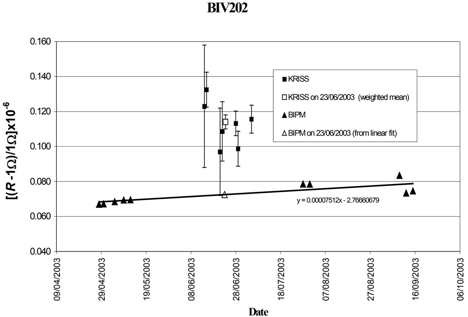
Figure 1. Relative deviation from the nominal 1  $\Omega$  value of the resistance of BIV202 vs time: a linear least-squares fit to the BIPM measurements (full line) and the weighted mean of the KRISS measurements. Uncertainty bars correspond to standard uncertainties of type A only. For each individual BIPM result, the type A standard uncertainty is about 3 parts in  $10^9$ .
