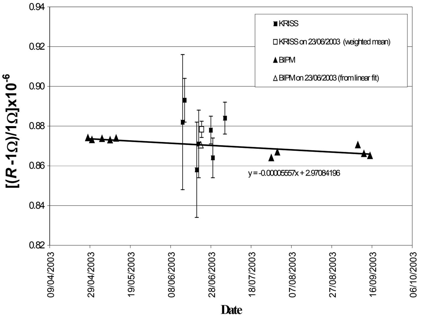
Figure 3. Relative deviation from the nominal 1  $\Omega$  value of the resistance of BIV205 vs time: a linear least-squares fit to the BIPM measurements (full line) and the weighted mean of the KRISS measurements. Uncertainty bars correspond to standard uncertainties of type A only. For each individual BIPM result, the type A standard uncertainty is about 3 parts in  $10^9$ .
