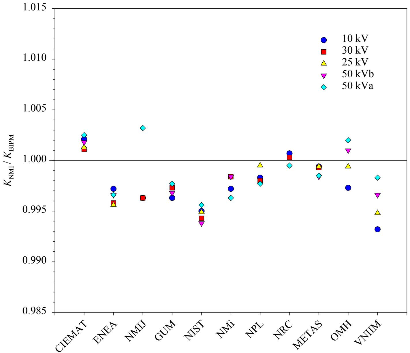
Figure 2. Results of BIPM low-energy x-ray comparisons, expressed as the ratio of the air-kerma rate determined by the standard of the national metrology institute (NMI) to that determined by the BIPM standard. For NMIs that have compared more than once at the BIPM, only the results of the most recent comparison are included.
