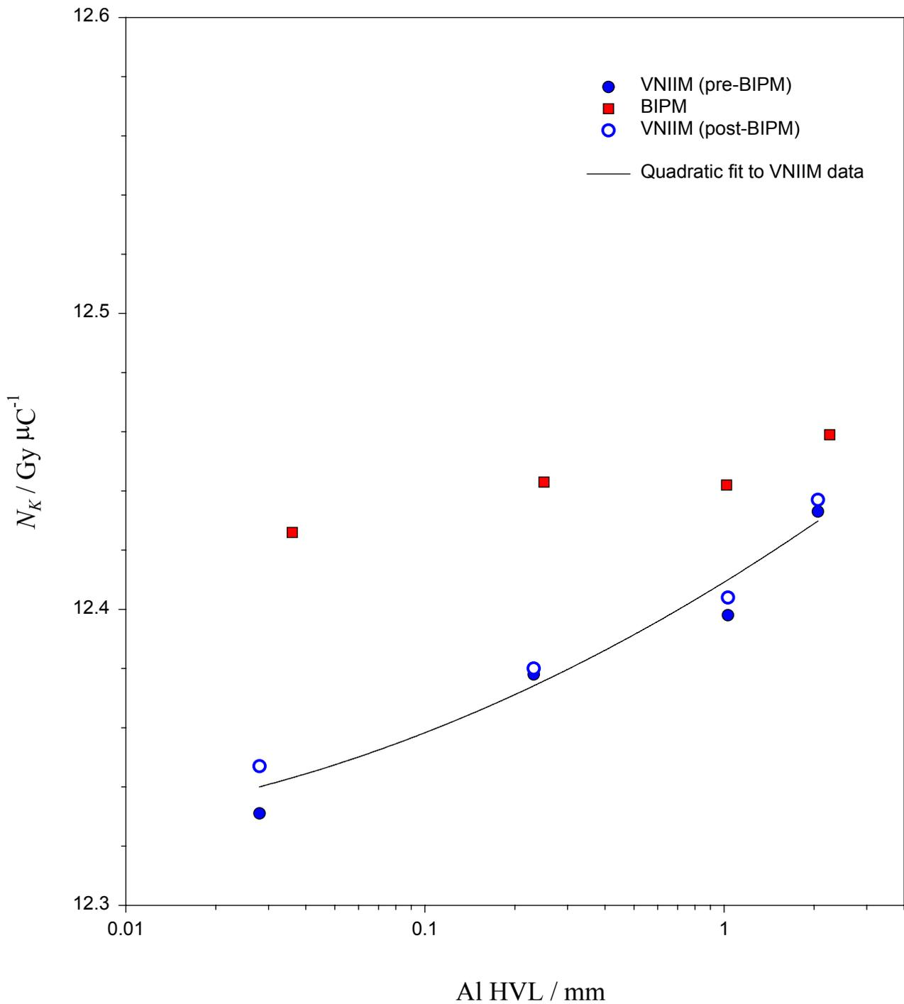
Figure 1. Results for the calibration coefficient  $N_K$  for transfer chamber IK10-60/2 at the BIPM and at the VNIIM, as a function of HVL. The line is a quadratic fit to the VNIIM data (open and closed circles) and is used to derive radiation quality correction factors  $k_Q$  (see text).
