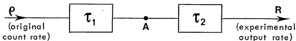
Fig. 1 - The notation used for the count rates in a series arrangement of two dead times. For measuring  $\tau_1$ , the statistical properties of the process are studied at A.
