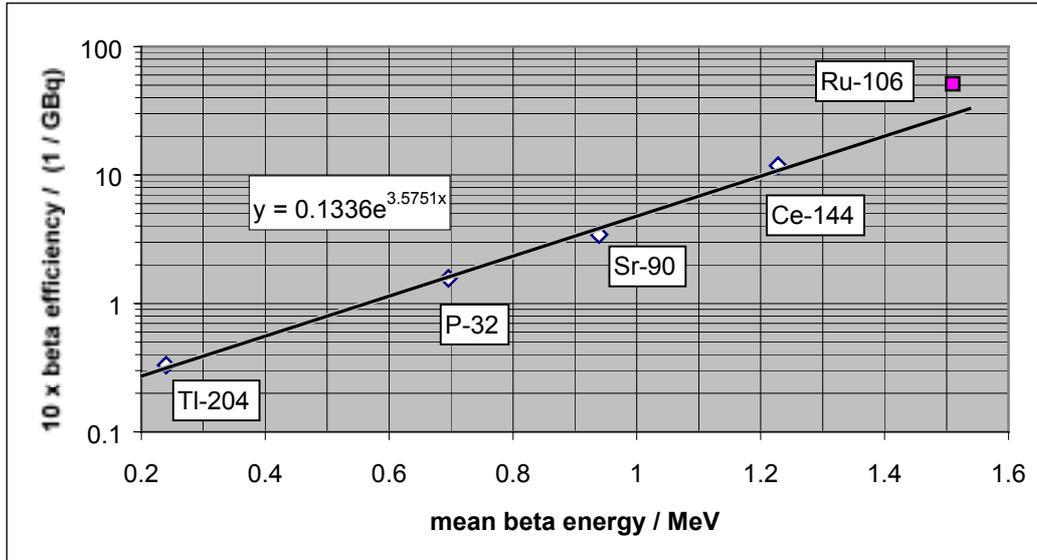
Figure 1: beta efficiency curve of the SIR ionization chamber. The full line is a fit to the white data points.
