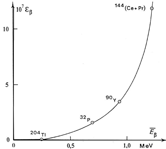
Figure 2: beta efficiency curve from (Rytz, 1985).
