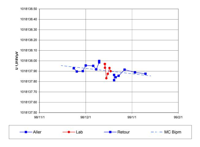
Figure 2. Values of the 1.018 V output of BIPM5 during the comparison: Corrections for temperature and pressure have been applied. The dashed straight line indicates the result of a linear least-squares fit to the BIPM results.
