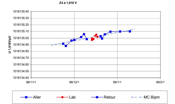
Figure 1 Values of the 1.018 V output of BIPM4 during the comparison: Corrections for temperature and pressure have been applied. The dashed straight line indicates the result of a linear least-squares fit to the BIPM results.
