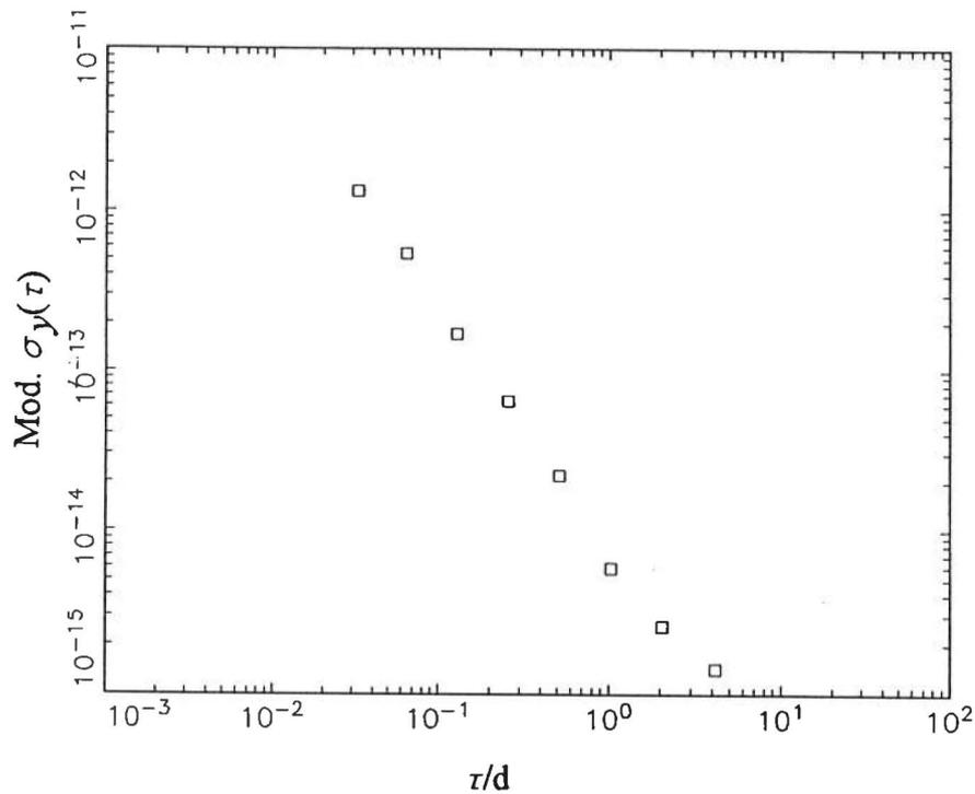
**Figure 1.** Square root of the modified Allan variance of the time series  $dt_{\text{OP}}$  for the period June 6-25, 1995.
