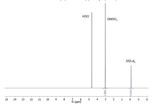
Figure 3 -  $^{1}$ H NMR spectrum of DSS- $d_{6}$  and DMSO<sub>2</sub> in D<sub>2</sub>O.
