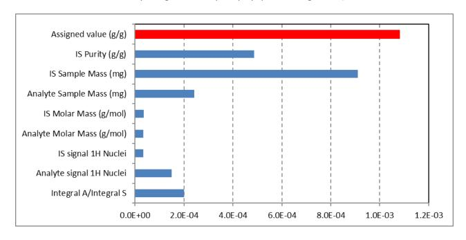
Figure 6 - Relative uncertainty components: MA assignment using DSS-d<sub>6</sub> in D<sub>2</sub>O
