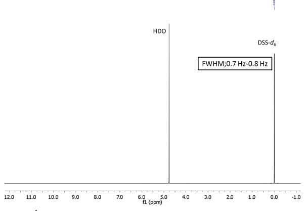
$^{1}$ H NMR spectrum of DSS- $d_{6}$  in D $_{2}$ O: JEOL ECS-400 spectrometer with Royal probe.
