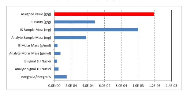
Figure 4 - Relative uncertainty components: DMSO<sub>2</sub> assignment using DSS-d<sub>6</sub> in D<sub>2</sub>O.
