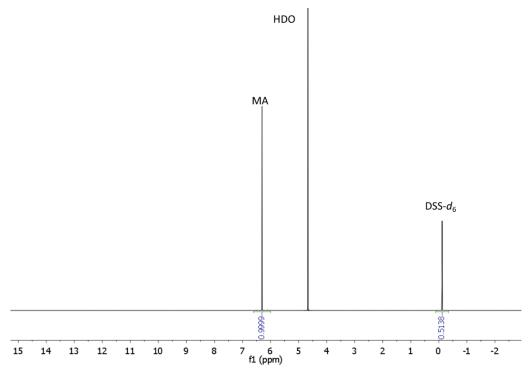
Figure 5 -  $^{1}$ H NMR of DSS- $d_{6}$  and MA in D<sub>2</sub>O.
