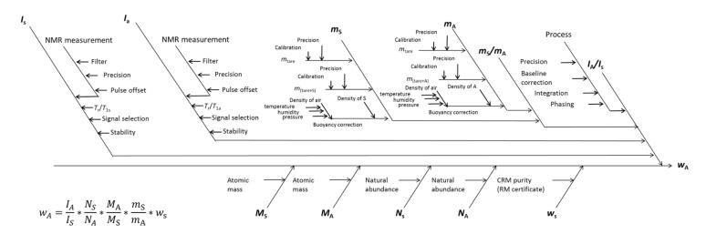
Figure 2 – Ishikawa diagram for input quantities considered for the measurement uncertainty estimation by qNMR
