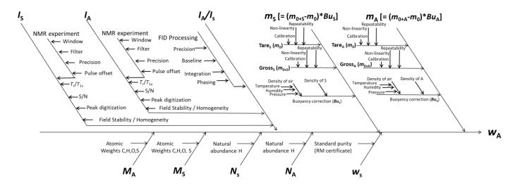
Figure 2 – Ishikawa diagram for input quantities considered for estimation of the measurement uncertainty of a purity assignment by qNMR
