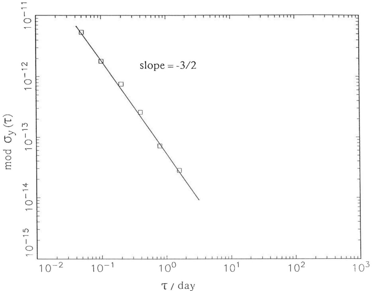
Figure 1. Square root of the modified Allan variance of the differences  $dt(i)_{NBS184} = [UTC(CRL) - GPS\ time(i)]_{Sony} - [UTC(CRL) - GPS\ time(i)]_{NBS184}$  for the period February 8-13, 1992.
