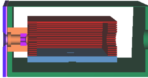
Fig.2. A cut-away of the geometry used for Monte Carlo simulations, created using the PENGEO code of PENELOPE [2].
