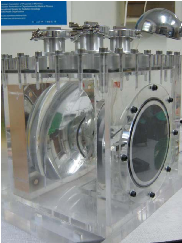
Fig. 6-c. The graphite window is seen to the right, covered by the PMMA window. Four vacuum flanges on the lid of the vacuum container allow the passage of electrical signals.
