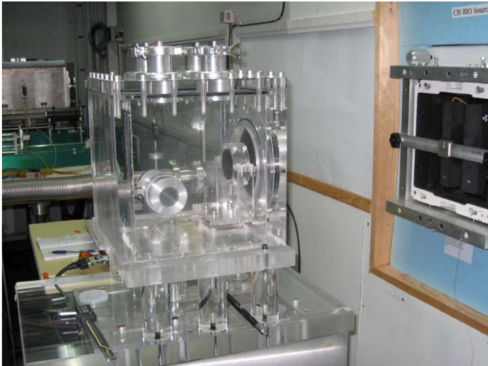
Figure 3. Calorimeter vacuum container made in PMMA, without reflectors inside.
