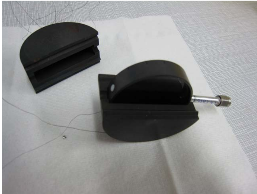
Figure 2. The graphite jacket shown now with the parallel-plate transfer ionization chamber.
