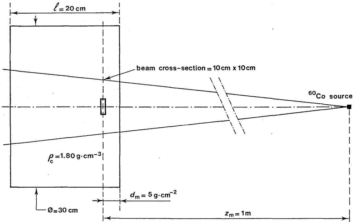
Fig. 1 - Geometrical conditions chosen for the comparisons.
