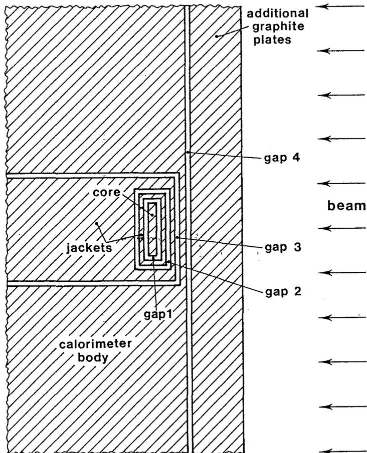
Fig. 2 - Schematic view of the gaps in a calorimeter.
