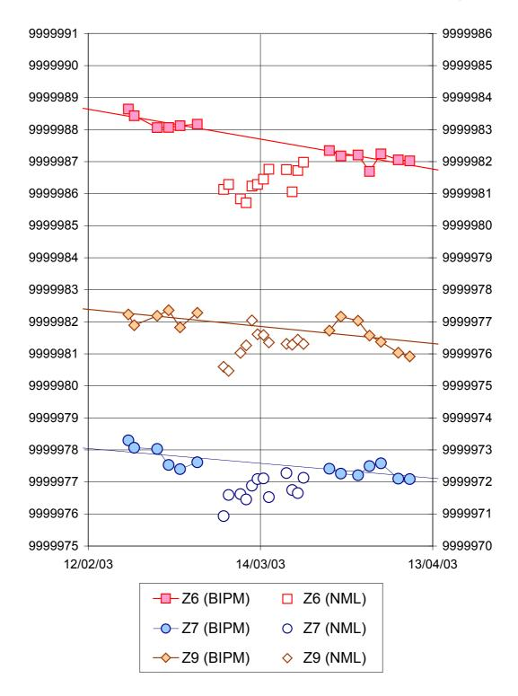
Figure 1. Voltage of BIPM6, BIPM7 and BIPM9 as a function of time, with linear least-squares fits (lsf) to the measurements of the BIPM
