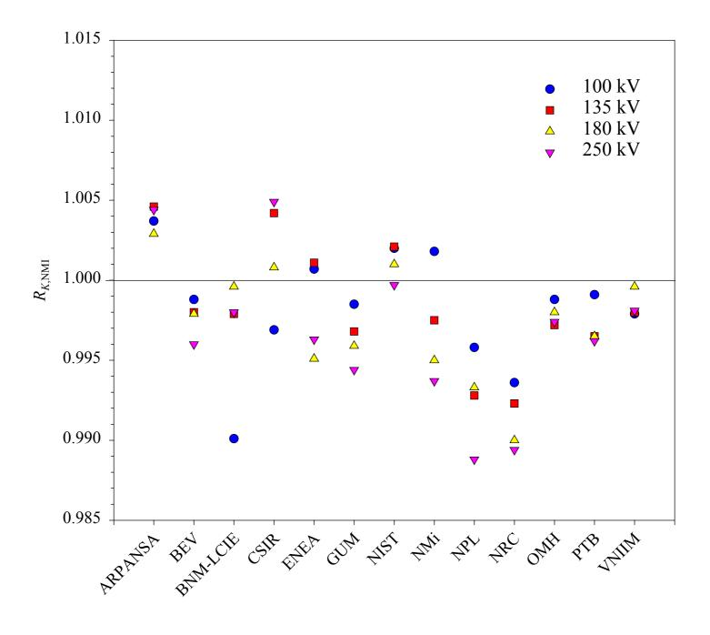
Figure 2. Results of BIPM medium-energy x-ray comparisons, expressed as the ratio  $R_{K,\text{NMI}}$  of the air-kerma rate detemined by the standard of the national metrology institute (NMI) to that determined by the BIPM standard. For NMIs that have compared more than once with the BIPM, only the results of the most recent comparison are included.
