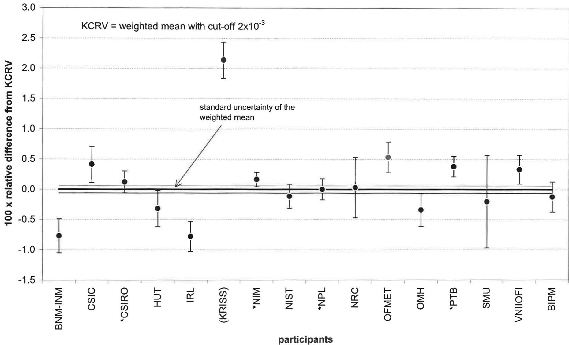
Figure 11: Results of the comparison averaged over all photometers per laboratory. The graph shows the relative difference from the weighted mean in percent for each laboratory. The uncertainties correspond to the standard uncertainties ( $k=1$ ) stated by the laboratories and do not include the uncertainty of the comparison itself.
