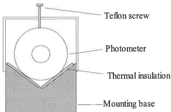
Figure 1: Thermal insulation of the photometer mount.
