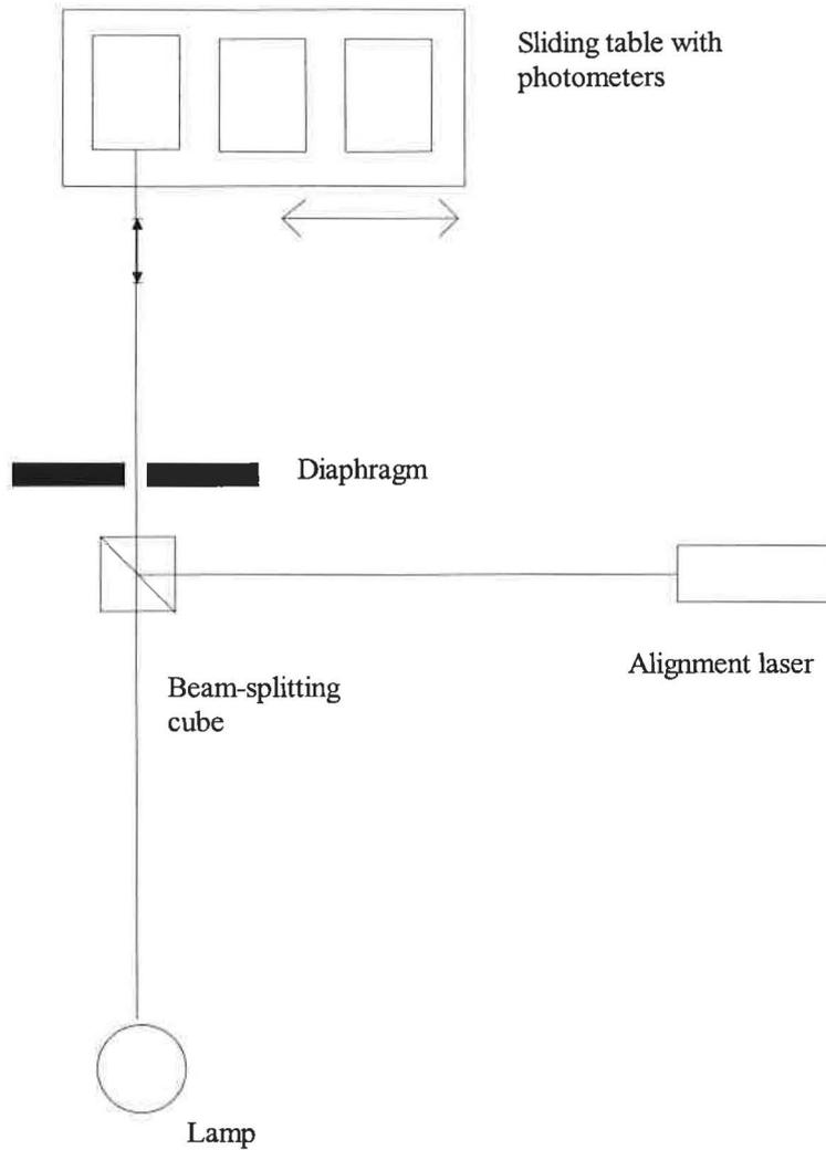
**Figure 9:** Photometer alignment.
