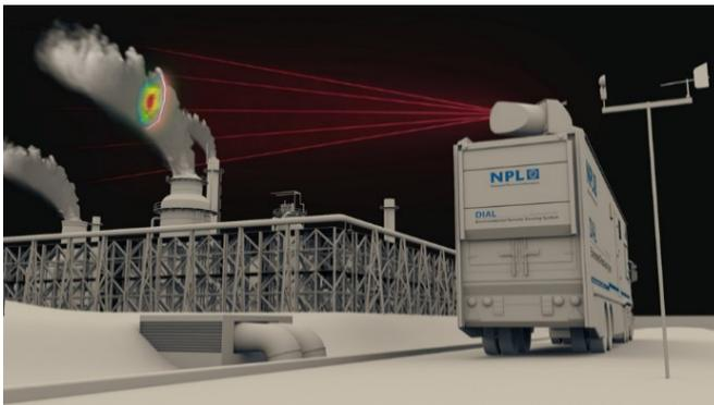
Figure 8: This figure illustrates an innovative method for measuring greenhouse gas (GHG) emission fluxes and concentrations, by using new sensing approaches. The image displays a mobile Differential Absorption Lidar (DIAL) facility for scanning emissions from chimneys. This system can monitor atmospheric pollutants remotely, at ranges of up to 1 km. DIAL measurements are real-time, directly traceable to primary standards of gas concentration and are free from interference and contamination.
