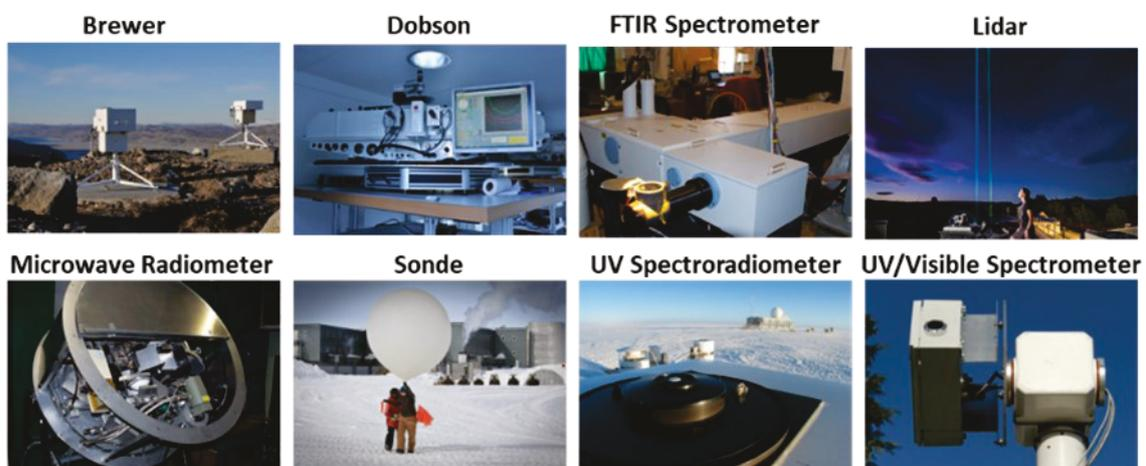
Figure 1: This figure shows a set of instruments used by the Network for the Detection of Atmospheric Composition Change (NDACC), a global network consisting of over 70 ground-based remote-sensing research stations with over 160 active instruments. NDACC plays a crucial role in the World Meteorological Organization's (WMO) Global Atmosphere Watch (GAW) Programme and is a significant component of the Integrated Global Atmospheric Chemistry Observation (IGACO) initiative.
