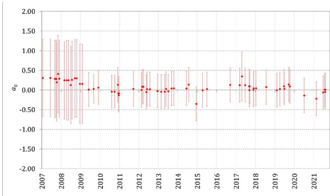
**Figure 2 : Intercept of the linear relationship between SRP28 and SRP27 obtained for each of the BIPM.QM-K1 comparisons realized at the BIPM. Uncertainties are calculated at  $k = 2$ , with the uncertainty budget in use at the time of each comparison.**
