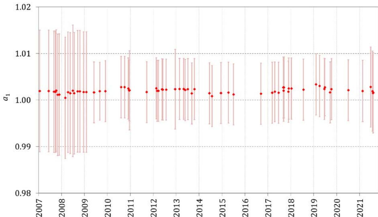
**Figure 1 : Slope of the linear relationship between SRP28 and SRP27 obtained for each of the BIPM.QM-K1 comparisons realized at the BIPM. Uncertainties are calculated at  $k = 2$ , with the uncertainty budget in use at the time of each comparison.**
