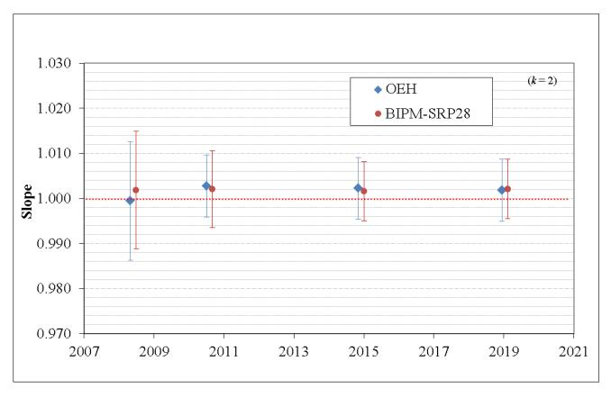
Figure 2: Results of the comparisons between SRP27, SRP28 and OEH SRP21 performed at the BIPM during the course of the key comparison BIPM.QM-K1. Uncertainties are calculated at k=2, with the uncertainty budget in use at the time of each comparison.
