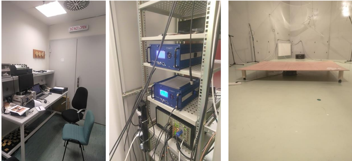
Fig.8 Measurement chain: left: Control Room – Middle: Pulse analyzer & Power amplifier – Right: Turntable and base plate
